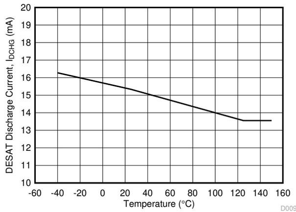
图 6-30.  $I_{DCHG}$  DESAT Discharge Current vs Temperature
