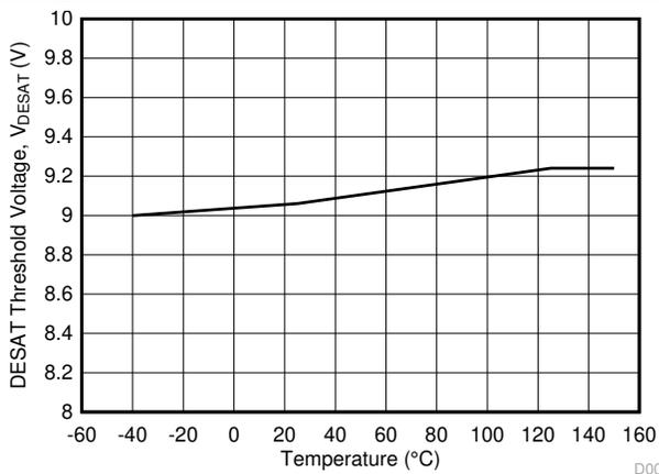
图 6-24.  $V_{DESAT}$  DESAT Threshold Voltage vs Temperature
