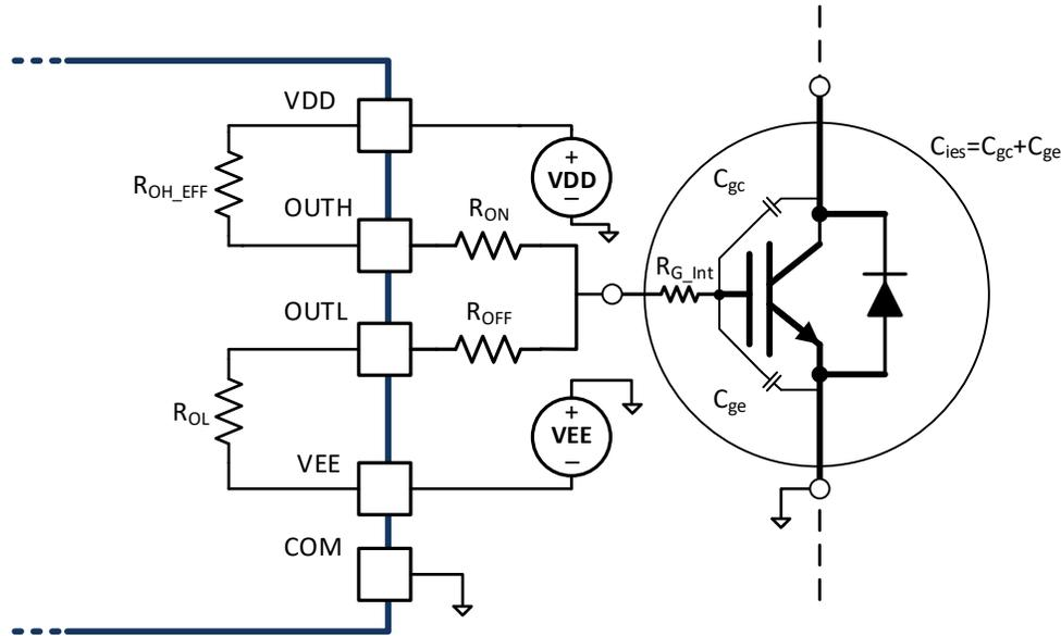
图 9-5. Output Model for Calculating Peak Gate Current
