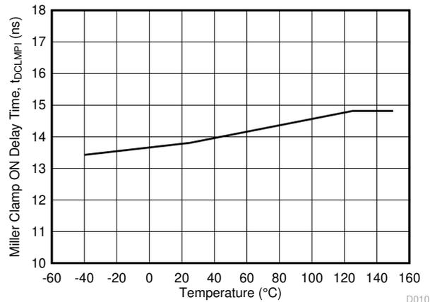
图 6-23.  $t_{DCLMPl}$  Miller Clamp ON Delay Time vs Temperature
