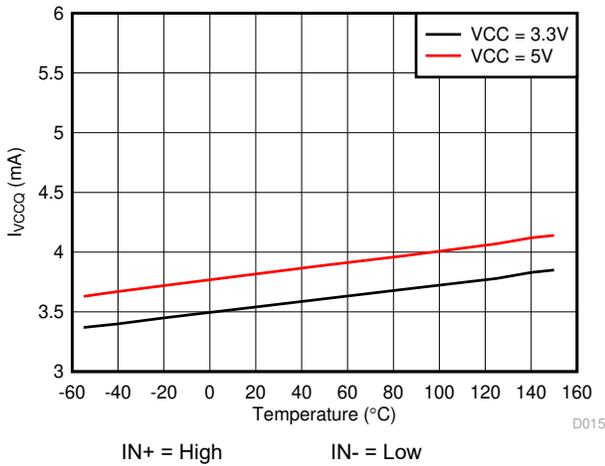
图 6-6. I<sub>VCCQ</sub> Supply Current vs Temperature
