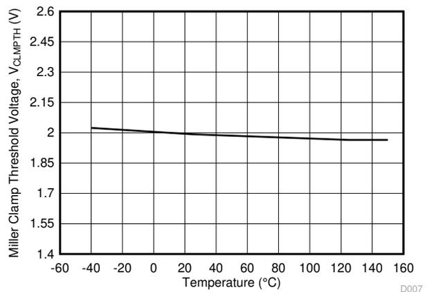
图 6-21.  $V_{CLMPH}$  Miller Clamp Threshold Voltage vs Temperature
