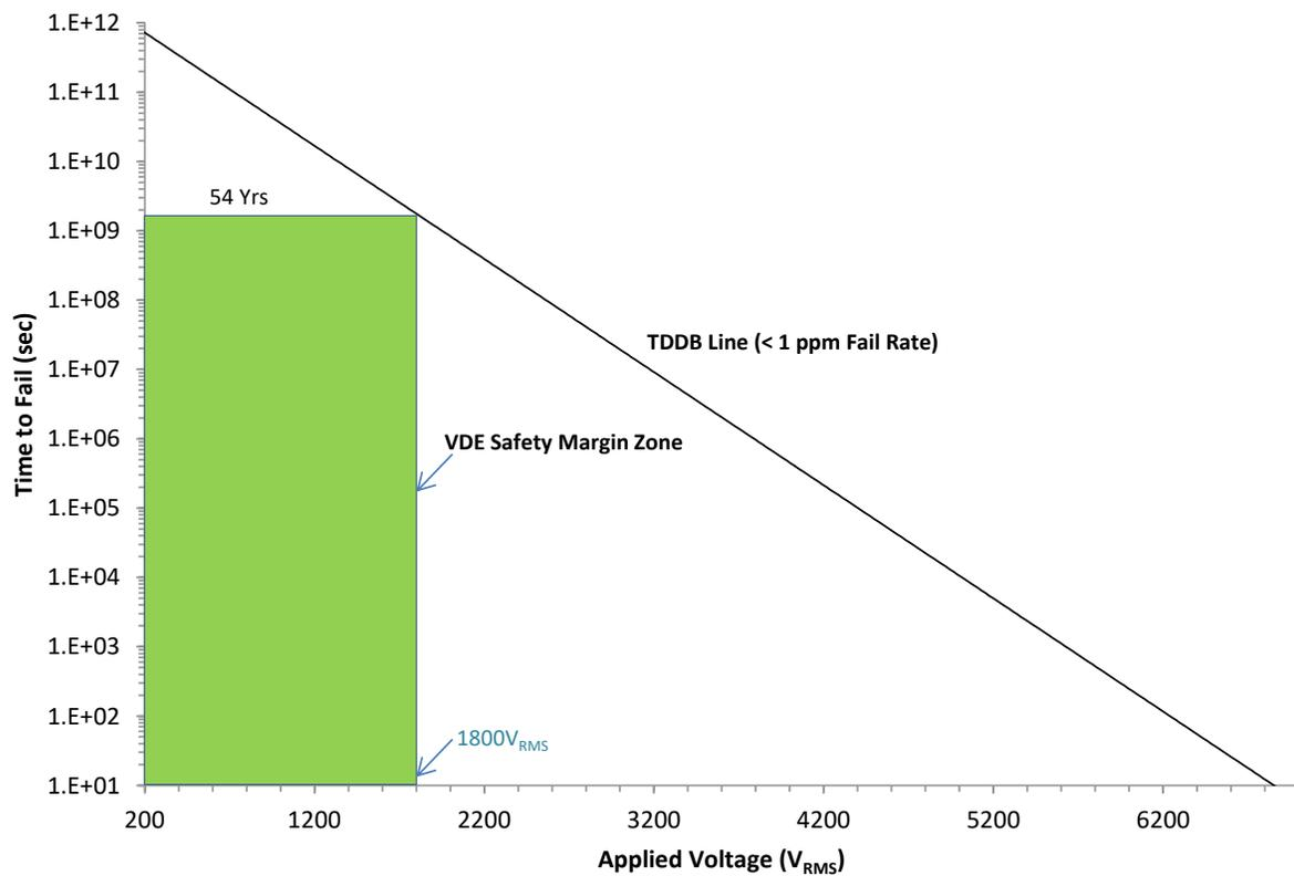
图 6-3. Reinforced Isolation Capacitor Life Time Projection
