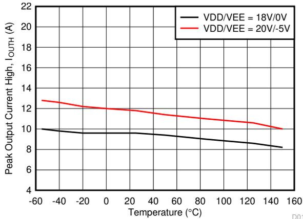
图 6-4. Output High Drive Current vs Temperature
