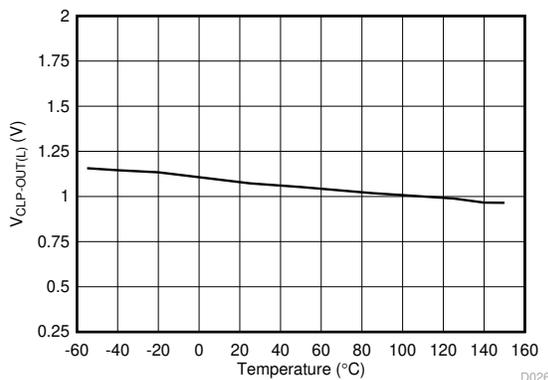
图 6-20.  $V_{CLP-OUT(L)}$  Short Circuit Clamping Voltage vs Temperature
