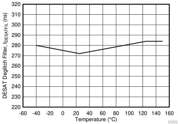
图 6-28.  $t_{DESATFIL}$  DESAT Deglitch Filter vs Temperature
