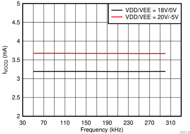
图 6-8. I<sub>VCCQ</sub> Supply Current vs Input Frequency
