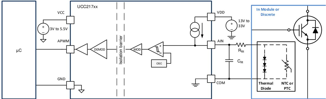
图 9-7. Thermal Diode or Thermistor Temperature Sensing Configuration
