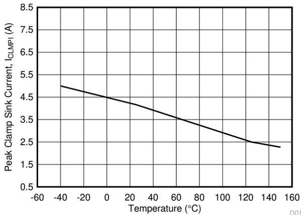
图 6-22.  $I_{CLMPl}$  Miller Clamp Sink Current vs Temperature
