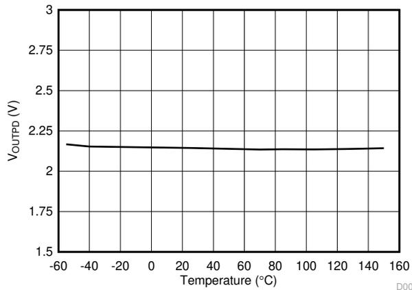
图 6-18.  $V_{OUTPD}$  Output Active Pulldown Voltage vs Temperature
