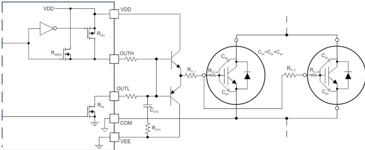
图 9-13. Current Buffer for Increased Drive Strength
