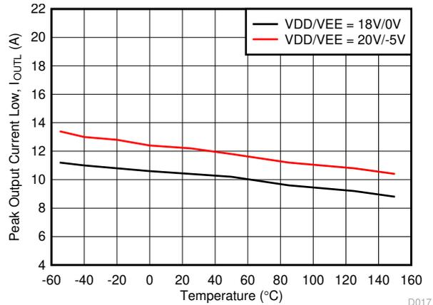
图 6-5. Output Low Driver Current vs Temperature
