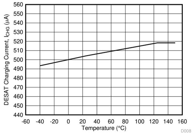
图 6-29.  $I_{CHG}$  DESAT Charging Current vs Temperature
