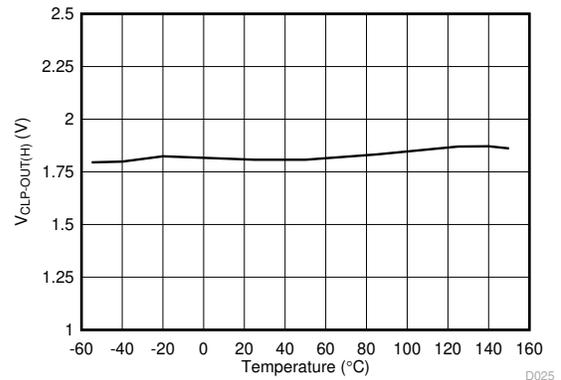
图 6-19.  $V_{CLP-OUT(H)}$  Short Circuit Clamping Voltage vs Temperature
