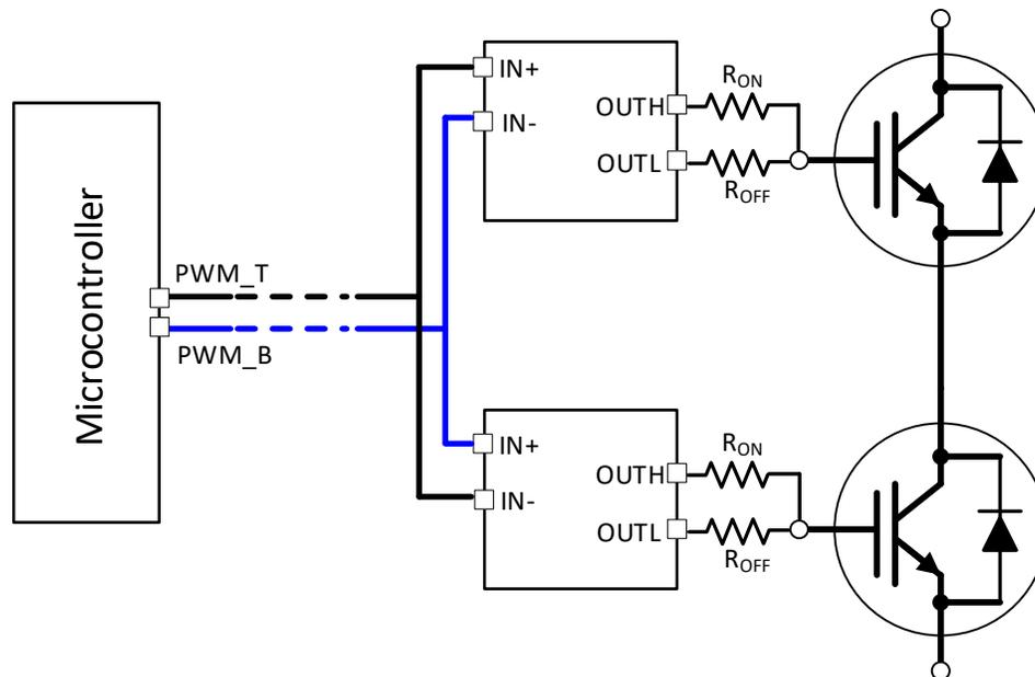
图 9-2. PWM Interlock for a Half Bridge
