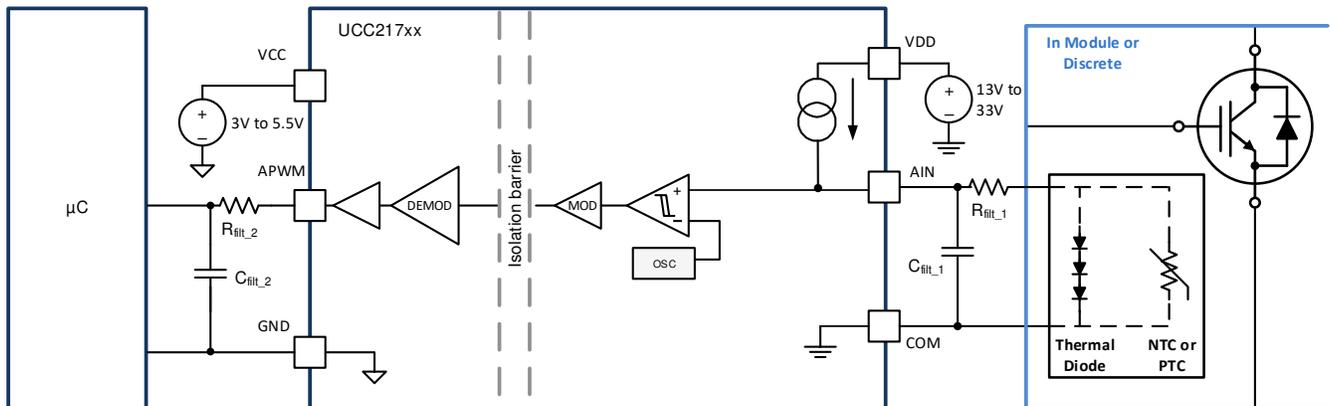
图 9-8. APWM Channel with Filtered Output
