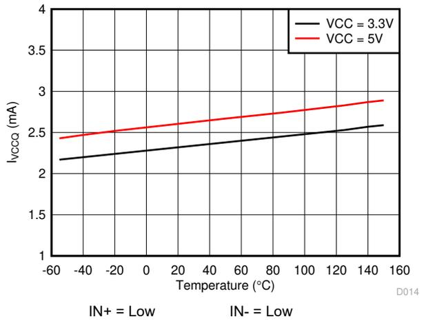
图 6-7. I<sub>VCCQ</sub> Supply Current vs Temperature
