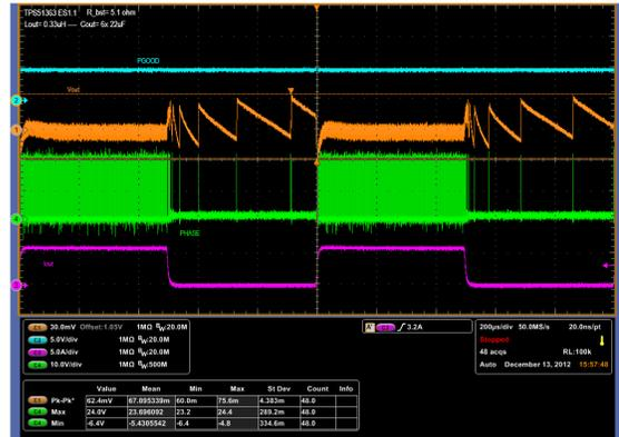
Figure 22.  $f = 800\text{kHz}$ ,  $V_{IN} = 20\text{V}$ ,  $I_{OUT} = 0\text{--}6\text{A}$
