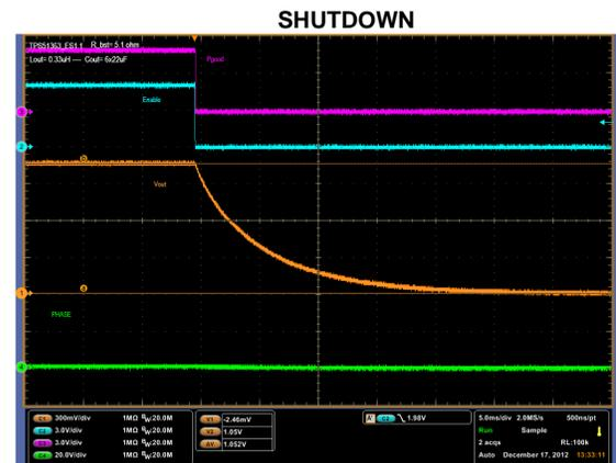
Figure 26.  $f = 800\text{kHz}$ ,  $V_{IN} = 20\text{V}$ ,  $I_{OUT} = 0\text{A}$
