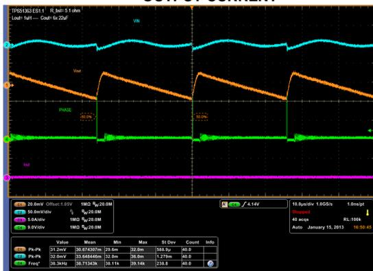
Figure 17.  $f = 400\text{kHz}$ ,  $V_{\text{IN}} = 20\text{V}$ ,  $I_{\text{OUT}} = 0.1\text{A}$
