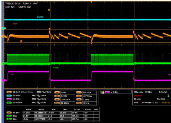
Figure 21.  $f = 400\text{kHz}$ ,  $V_{IN} = 20\text{V}$ ,  $I_{OUT} = 0\text{--}5\text{A}$
