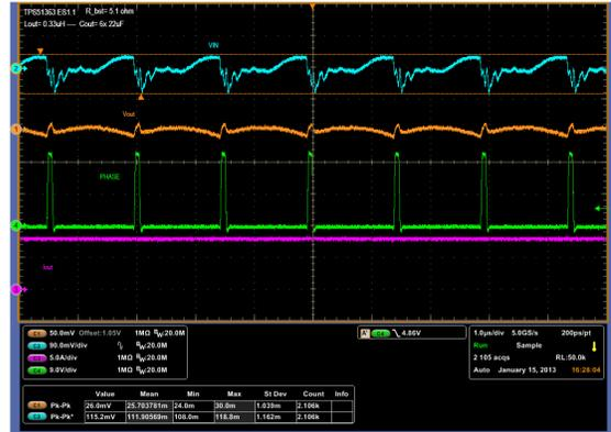
Figure 20.  $f = 800\text{kHz}$ ,  $V_{IN} = 20\text{V}$ ,  $I_{OUT} = 8\text{A}$
