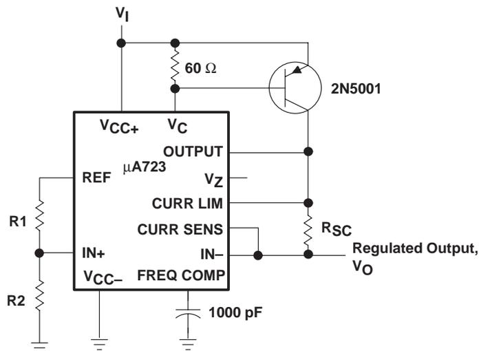
Figure 5. Positive-Voltage Regulator (External pnp Pass Transistor)
