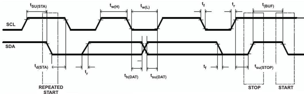
Figure 1. I<sup>2</sup>C-Compatible Interface Timing Diagrams
