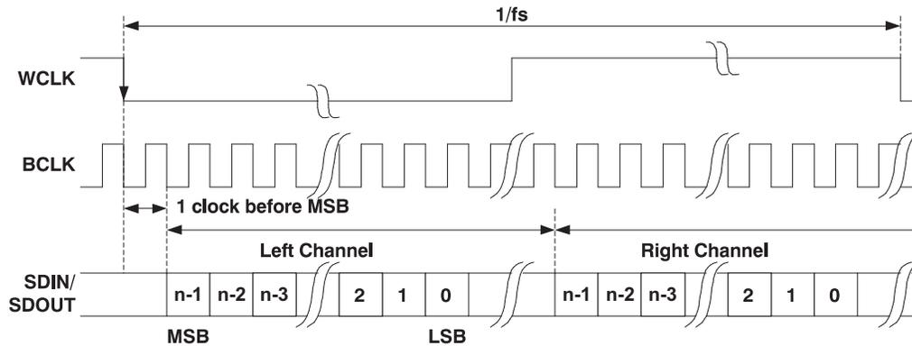
**Figure 35. I<sup>2</sup>S Serial Data Bus Mode Operation**
