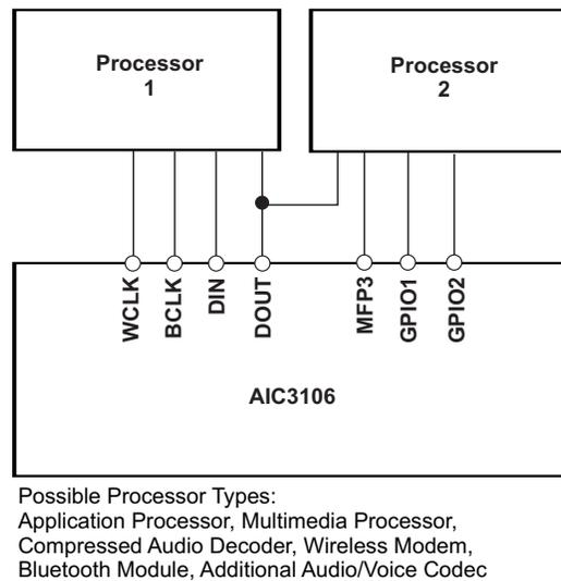
**Figure 32. TLV320AIC3106-Q1 Connected To Multiple Audio Devices**
