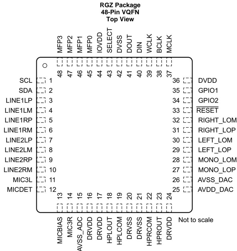
Solder the VQFN thermal pad to the ground plane (DRVSS).
