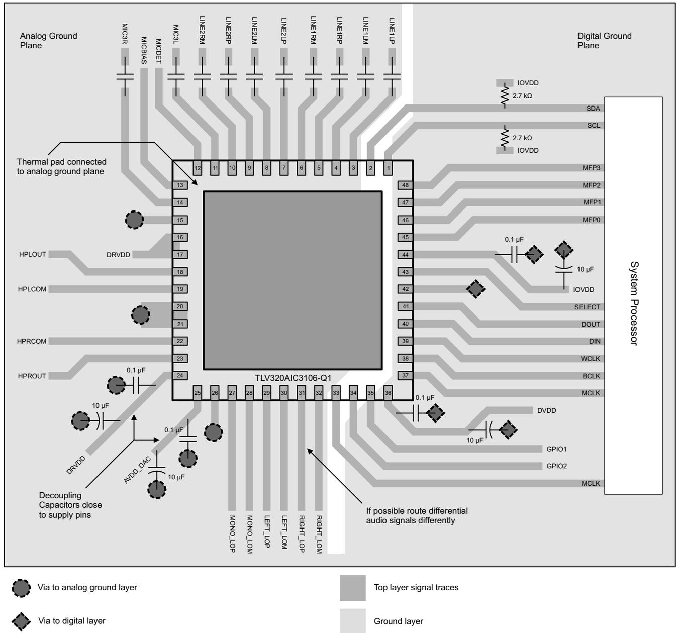
Figure 44. Layout Diagram
