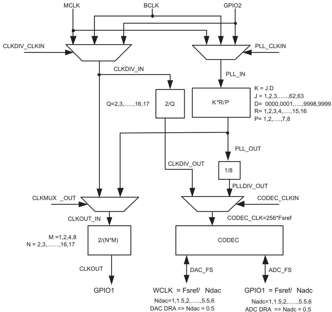
**Figure 38. Audio Clock Generation Processing**
