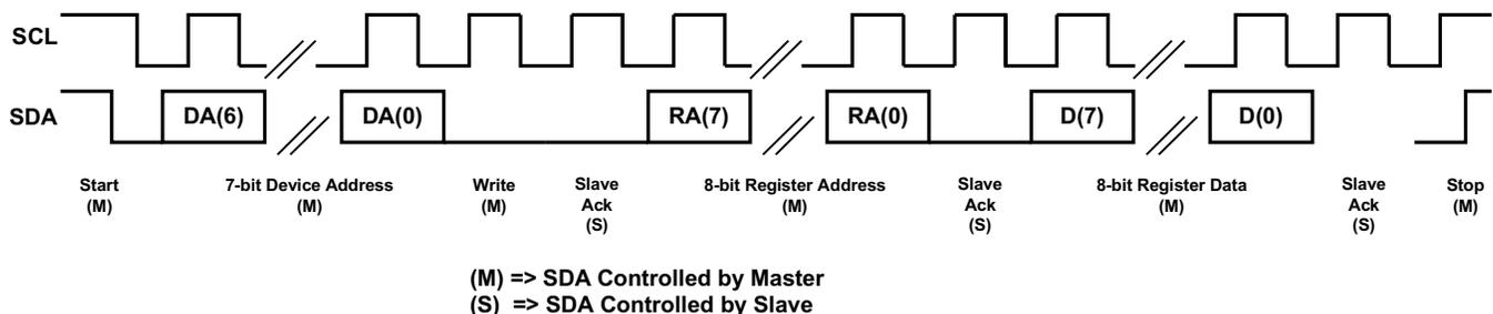
**Figure 29. I<sup>2</sup>C Write**
