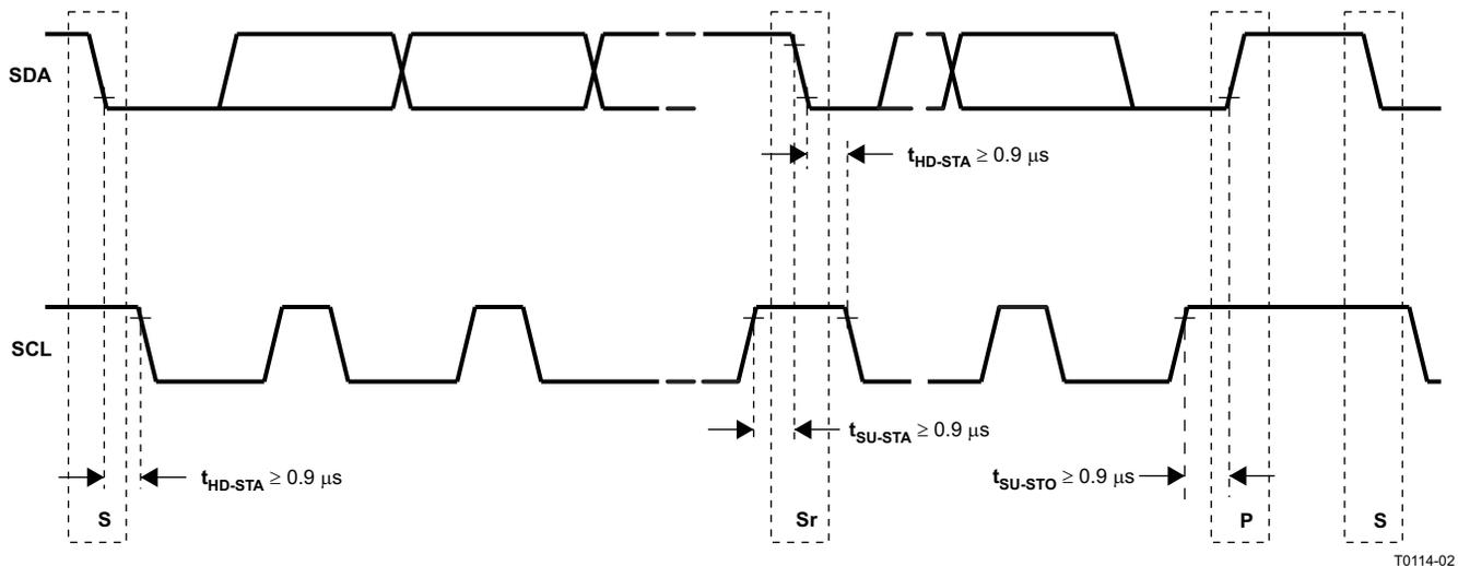
Figure 28. I<sup>2</sup>C Interface Timing
