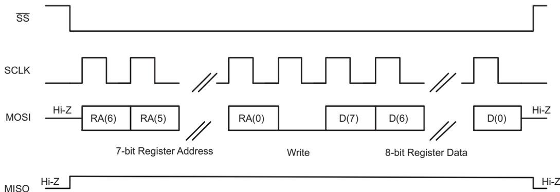
Figure 26. SPI Write
