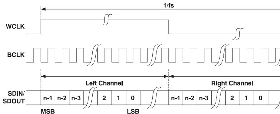
Figure 34. Left-Justified Serial Data Bus Mode Operation
