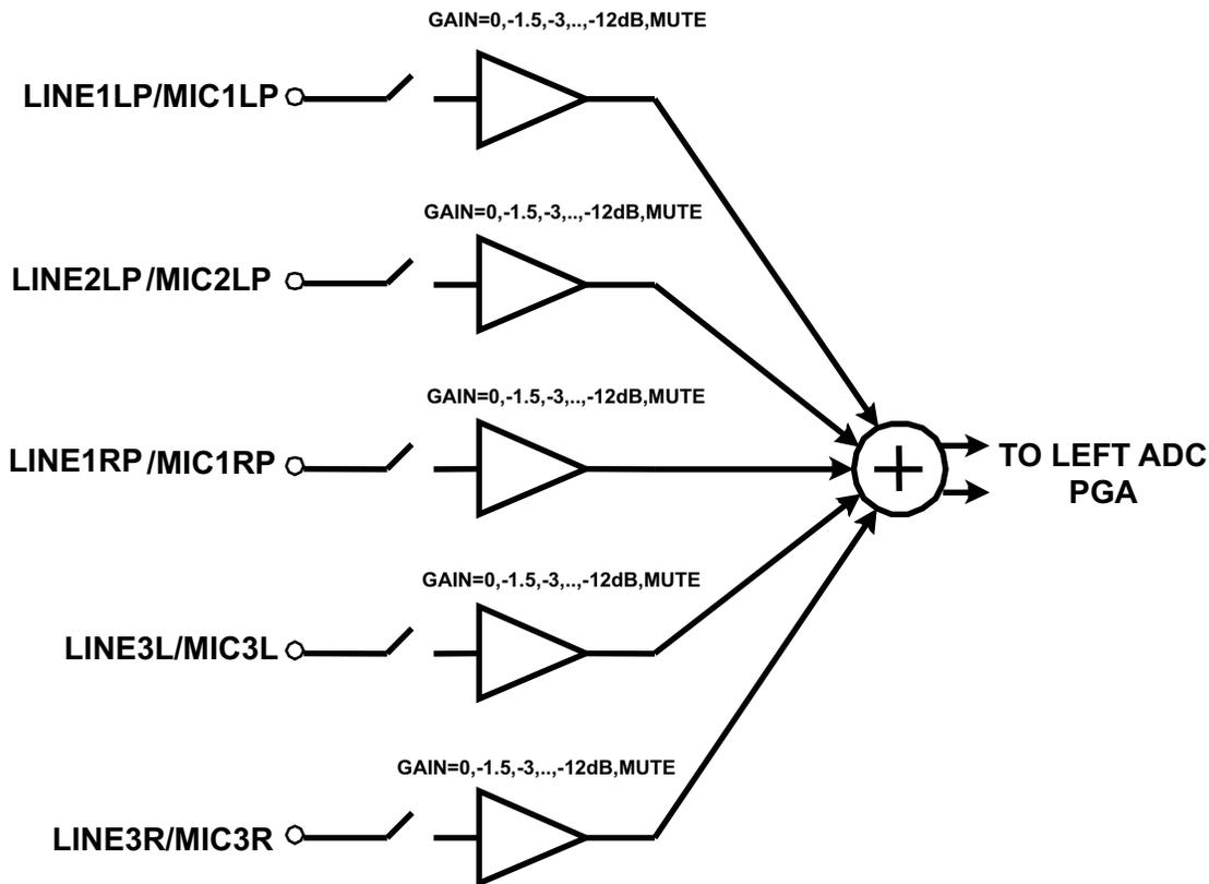
Figure 17. Left Channel Single-Ended Analog Input Mixing Configuration
