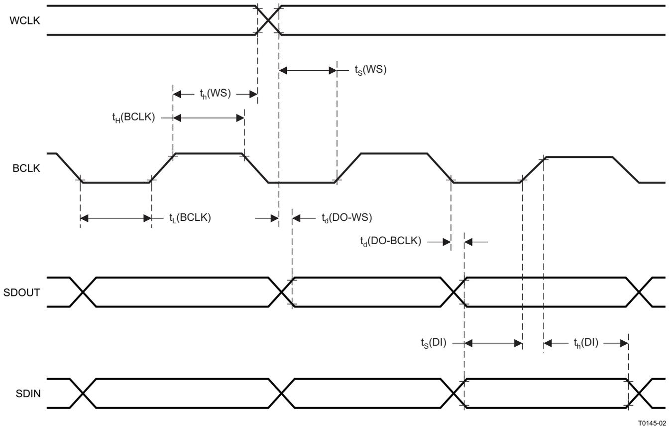
Figure 2. I<sup>2</sup>S/LJF/RJF Timing In Slave Mode
