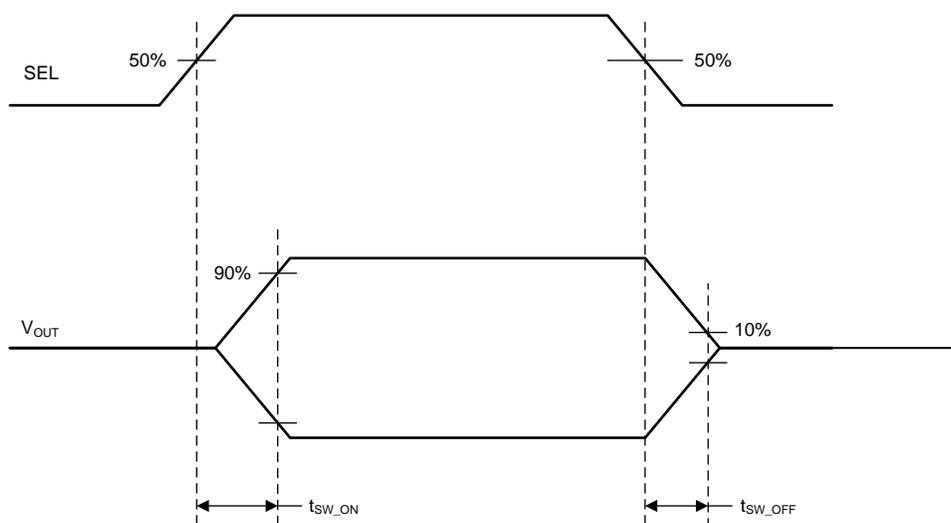
**Figure 2. Switch On and Off Timing Diagram**
