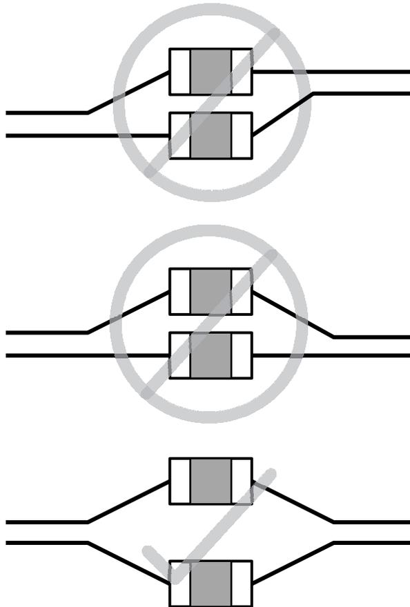
**Figure 19. AC-Coupling Placement**
