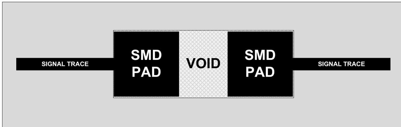
Figure 20. Reference Plane Voiding of Surface-Mount Devices
