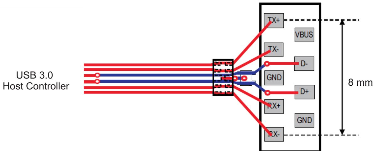
Figure 21. Flow-Through Routing
