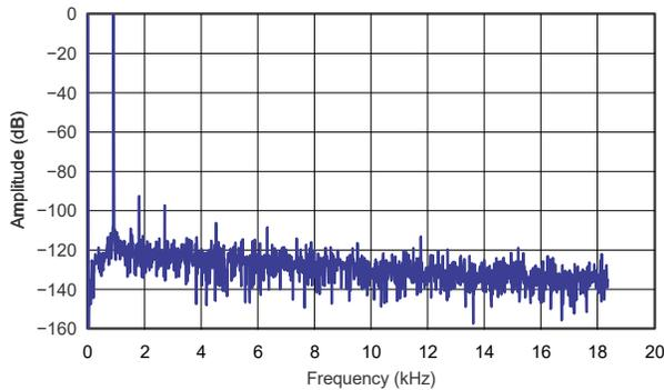
图 8-5. DAC to Line Output FFT Plot
