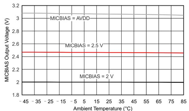
图 8-10. MICBIAS Output Voltage vs Ambient Temperature
