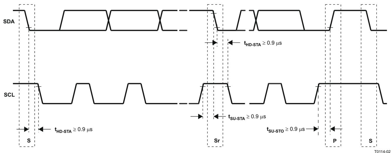
**图 9-13. I<sup>2</sup>C Interface Timing**
