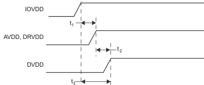
图 11-1. Power-Supply Sequencing
