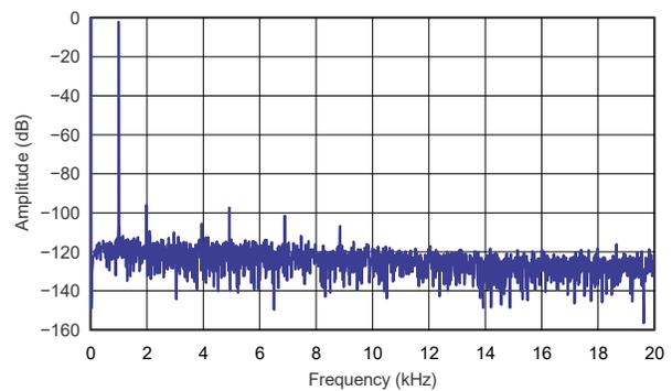
图 8-6. Line Input to ADC FFT Plot
