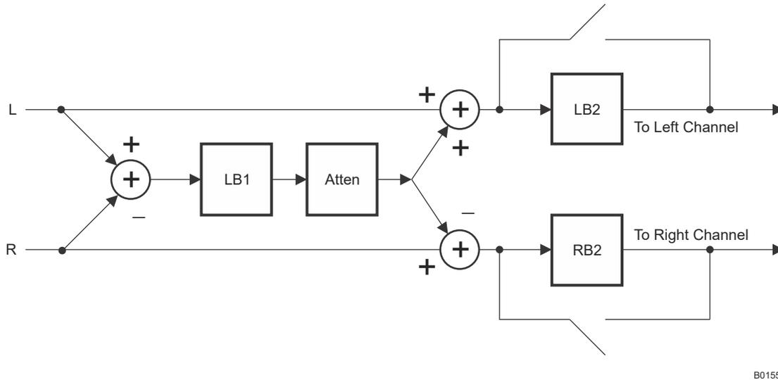
**图 9-3. Architecture of Digital Audio Processing With 3-D Effects Enabled**
