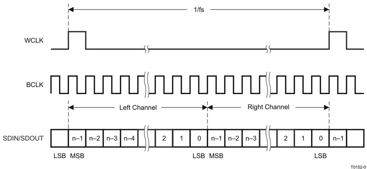
图 9-19. DSP Serial Data Bus Mode Operation
