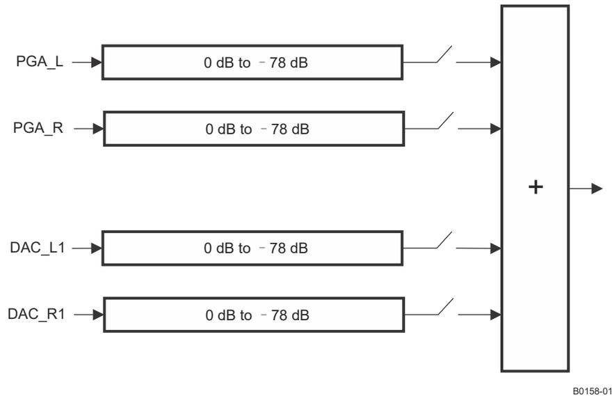
**图 9-6. Detail of Volume Control and Mixing Function**
