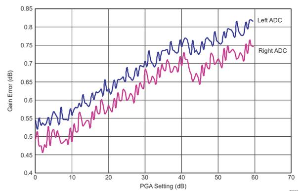
图 8-8. ADC Gain Error vs PGA Gain Setting
