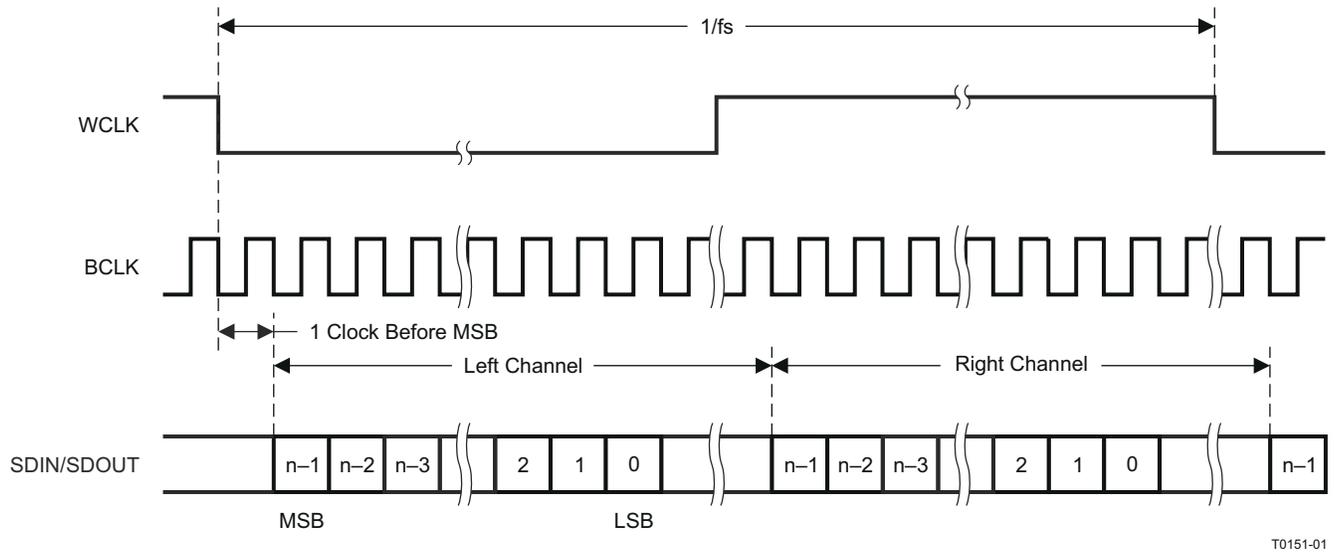
图 9-18. I<sup>2</sup>S Serial Data Bus Mode Operation
