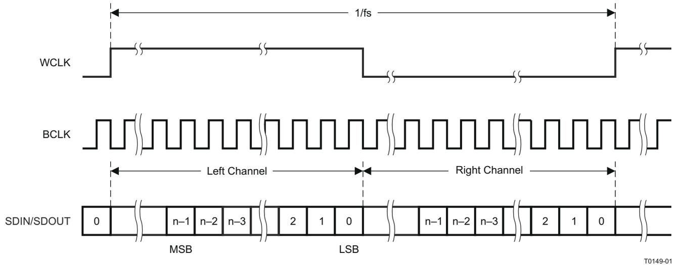
图 9-16. Right-Justified Serial Data Bus Mode Operation
