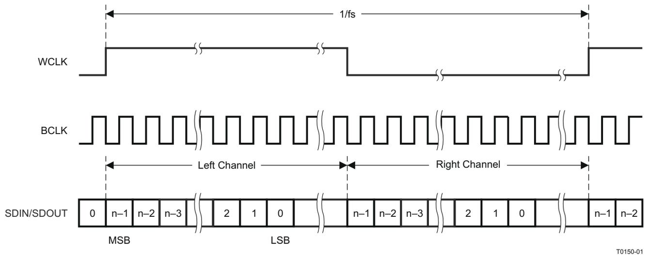
图 9-17. Left-Justified Serial Data Bus Mode Operation
