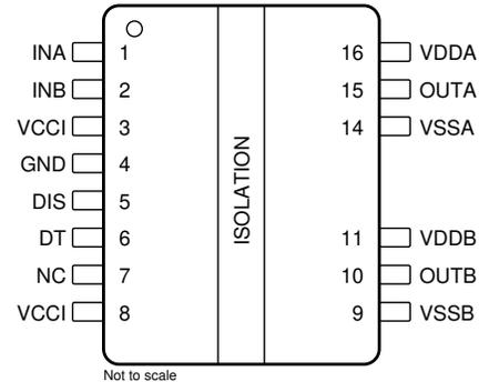
Figure 6-2. DWK Package 14-Pin SOIC Top View
