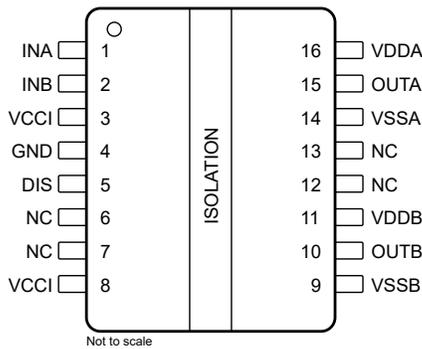
Figure 6-3. DW Package 16-Pin SOIC Top View
