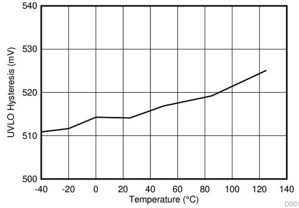
**Figure 7-15. 8-V VDD UVLO Threshold Hysteresis Voltage**
