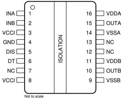
Figure 6-1. DW Package 16-Pin SOIC Top View
