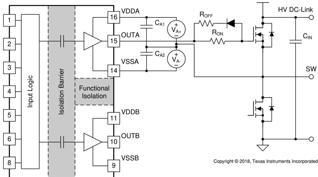
**Figure 10-3. Negative Bias with Two Iso-Bias Power Supplies**
