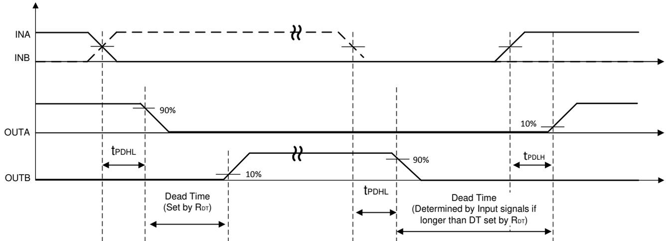
**Figure 8-6. Dead Time Switching Parameters for UCC21540/A, UCC21541**
