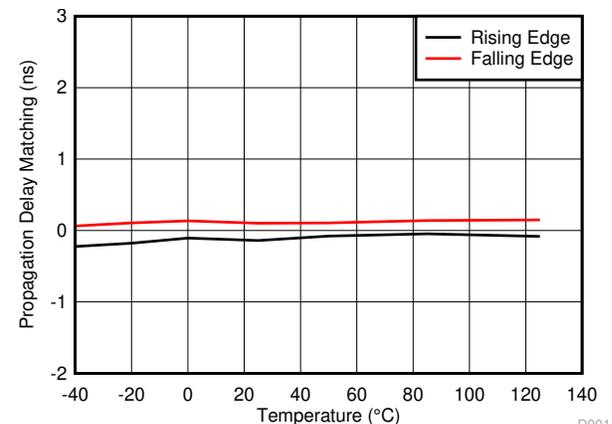
**Figure 7-19. Propagation Delay Matching, Rising and Falling Edge**
