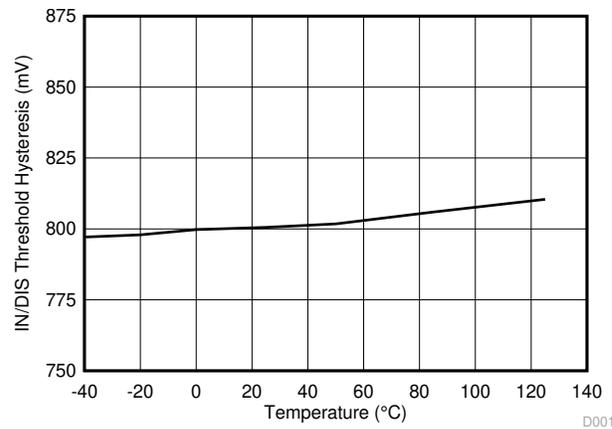
**Figure 7-17. INA/INB/DIS High and Low Threshold Hysteresis**
