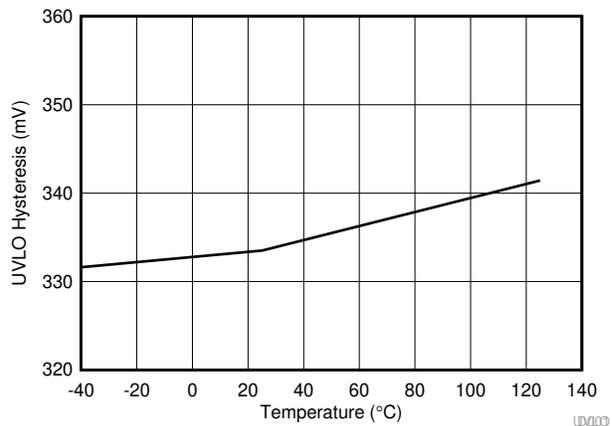
**Figure 7-13. 5-V VDD UVLO Threshold Hysteresis Voltage**
