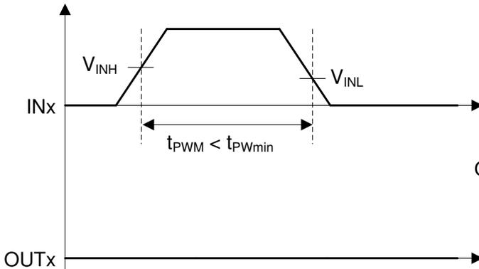
Figure 8-1. Deglitch Filter – Turn ON
