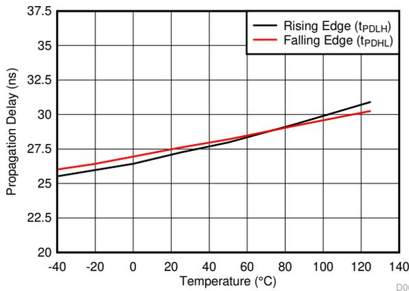
**Figure 7-18. Propagation Delay, Rising and Falling Edge**
