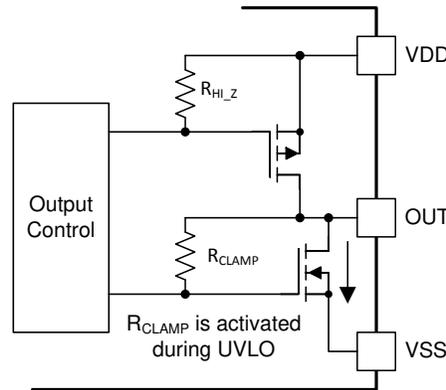
**Figure 9-1. Simplified Representation of Active Pull Down Feature**
