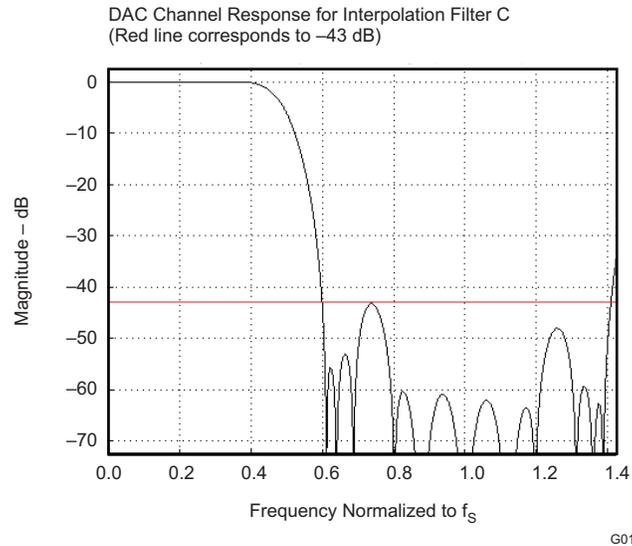
**Figure 5-16. Frequency Response of DAC Interpolation Filter C**
