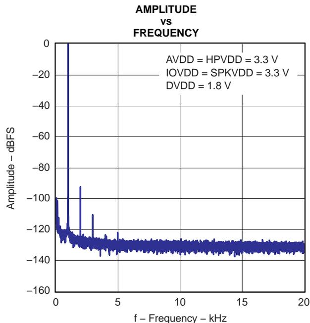
Figure 4-9. FFT - Line-In Bypass to Headphone Output
