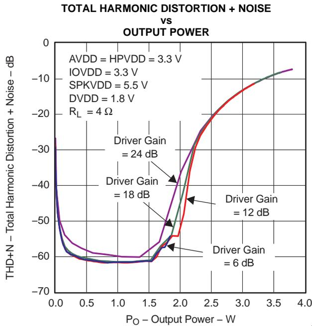
Figure 4-4. Max Class-D Speaker-Driver Output Power ( $R_L = 4 \Omega$ )
