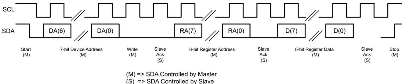
Figure 5-35. I<sup>2</sup>C Write
