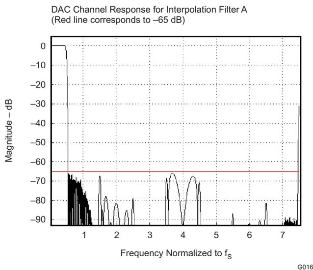
**Figure 5-14. Frequency Response of DAC Interpolation Filter A**
