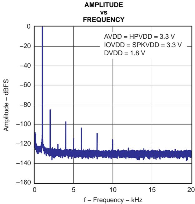
Figure 4-1. FFT - DAC to Line Output
