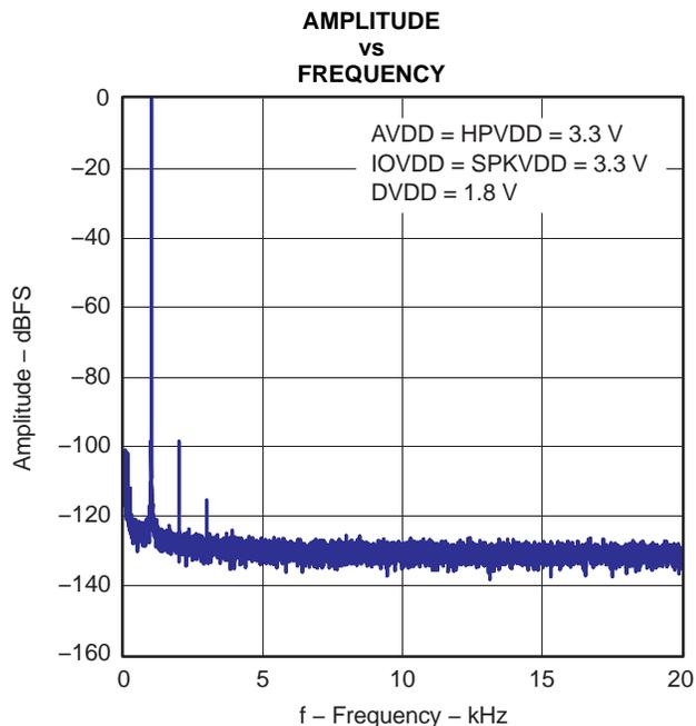
Figure 4-8. FFT - Line-In Bypass to Line Output
