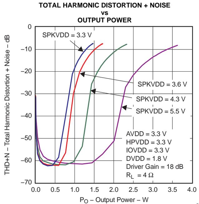
Figure 4-5. Class-D Speaker-Driver Output Power ( $R_L = 4 \Omega$ )
