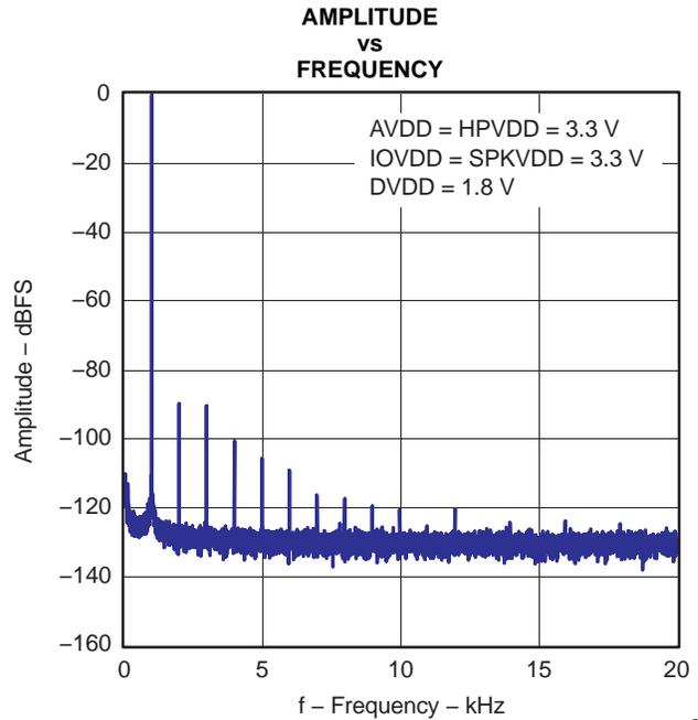
Figure 4-2. FFT - DAC to Headphone Output
