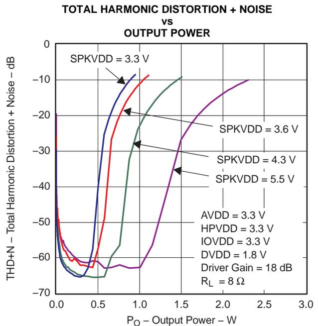
Figure 4-7. Class-D Speaker-Driver Output Power ( $R_L = 8 \Omega$ )
