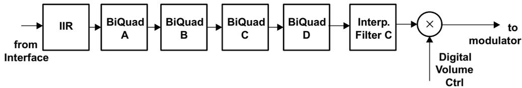
Figure 5-9. Signal Chain for PRB\_P19 and PRB\_P22
