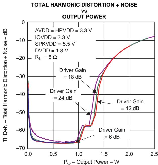
Figure 4-6. Max Class-D Speaker-Driver Output Power ( $R_L = 8 \Omega$ )
