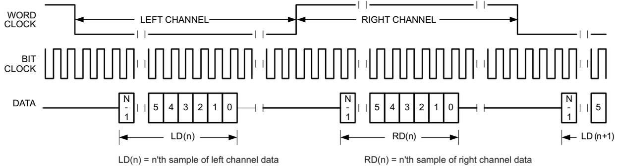
Figure 5-29. Timing Diagram for I²S Mode With Offset = 2
