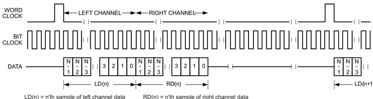
Figure 5-32. Timing Diagram for DSP Mode With Offset = 1
