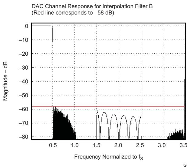
**Figure 5-15. Frequency Response of Channel Interpolation Filter B**
