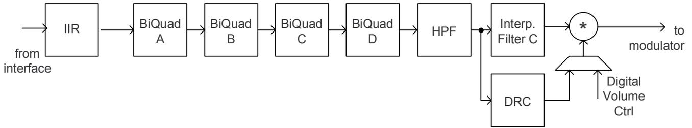
Figure 5-8. Signal Chain for PRB\_P18 and PRB\_P21
