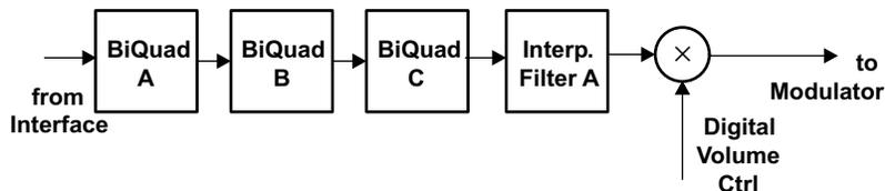
**Figure 5-2. Signal Chain for PRB\_P1 and PRB\_P4**
