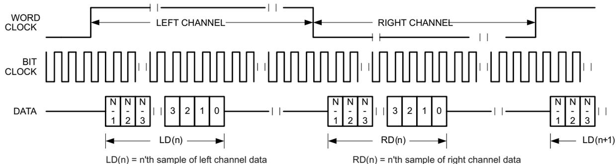
Figure 5-26. Timing Diagram for Left-Justified Mode With Offset = 1
