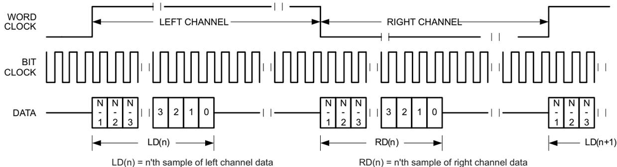
Figure 5-25. Timing Diagram for Left-Justified Mode
