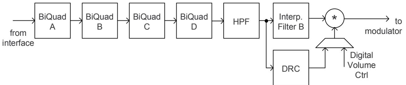
Figure 5-6. Signal Chain for PRB\_P8 and PRB\_P13
