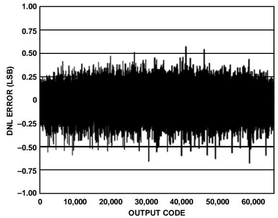
Figure 19. AD9268-80 DNL with  $f_{IN} = 9.7$  MHz
