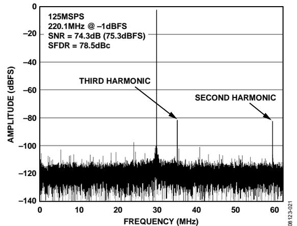
Figure 37. AD9268-125 Single-Tone FFT with  $f_{IN} = 220.1$  MHz
