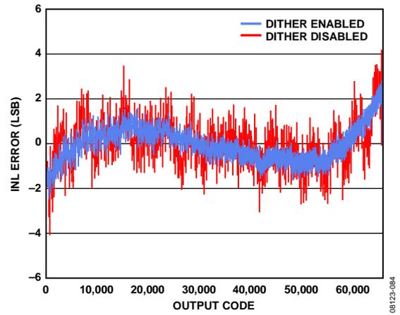
Figure 30. AD9268-105 INL with  $f_{IN} = 9.7$  MHz
