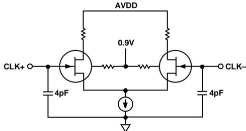
Figure 74. Equivalent Clock Input Circuit
