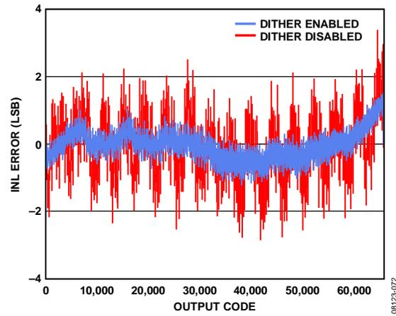
Figure 18. AD9268-80 INL with  $f_{IN} = 9.7$  MHz
