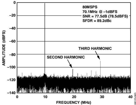
Figure 9. AD9268-80 Single-Tone FFT with  $f_{IN} = 70.1$  MHz
