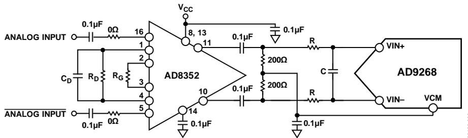
Figure 69. Differential Input Configuration Using the AD8352
