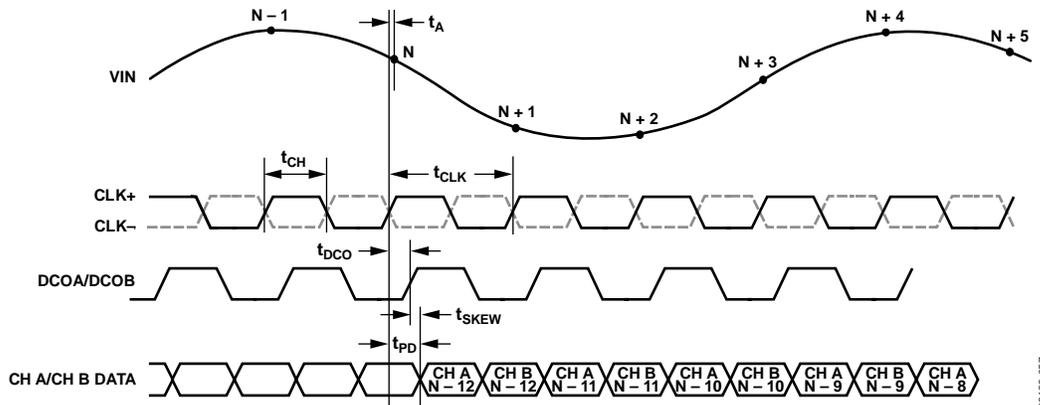
Figure 3. CMOS Interleaved Output Mode Data Output Timing
