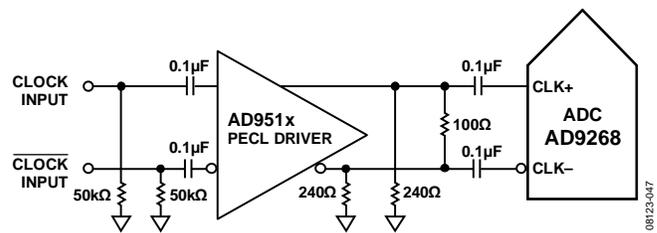
Figure 77. Differential PECL Sample Clock (Up to 625 MHz)
