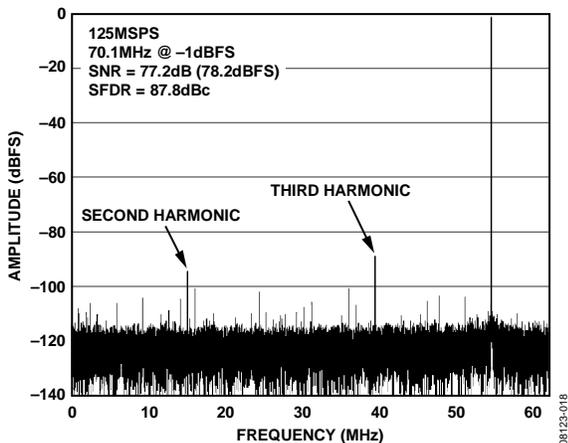
Figure 34. AD9268-125 Single-Tone FFT with  $f_{IN} = 70.1$  MHz
