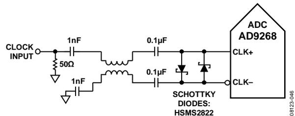
Figure 76. Balun-Coupled Differential Clock (Up to 625 MHz)
