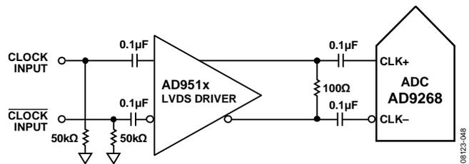
Figure 78. Differential LVDS Sample Clock (Up to 625 MHz)
