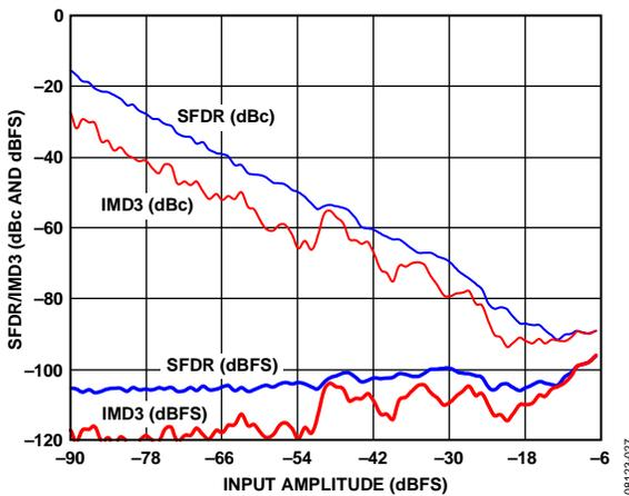
Figure 46. AD9268-125 Two-Tone SFDR/IMD3 vs. Input Amplitude ( $A_{IN}$ ) with  $f_{IN1} = 29.1$  MHz,  $f_{IN2} = 32.1$  MHz,  $f_s = 125$  MSPS
