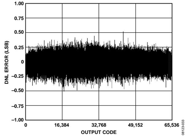
Figure 53. AD9268-125 DNL with  $f_{IN} = 9.7$  MHz
