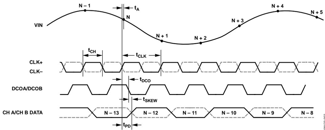
Figure 2. CMOS Default Output Mode Data Output Timing
