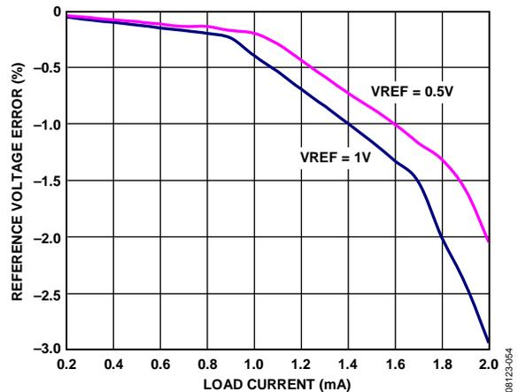
Figure 72. Reference Voltage Accuracy vs. Load Current
