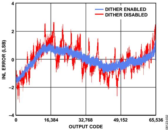
Figure 52. AD9268-125 INL with  $f_{IN} = 9.7$  MHz
