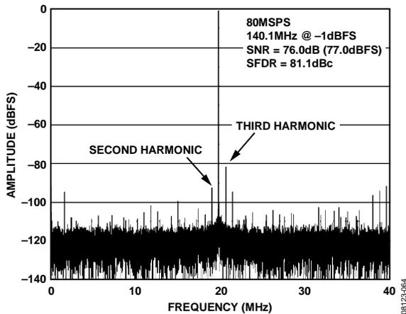
Figure 10. AD9268-80 Single-Tone FFT with  $f_{IN} = 140.1$  MHz
