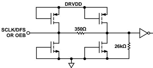
Figure 59. Equivalent SCLK/DFS or OEB Input Circuit
