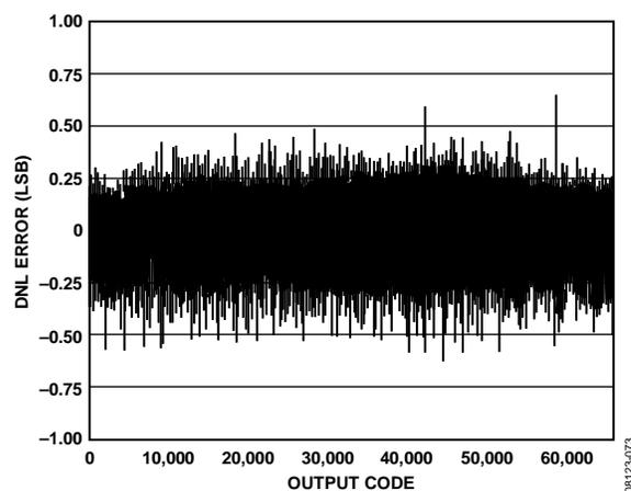
Figure 31. AD9268-105 DNL with  $f_{IN} = 9.7$  MHz
