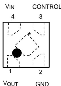
\*Center electrode should be connected to GND or Open
