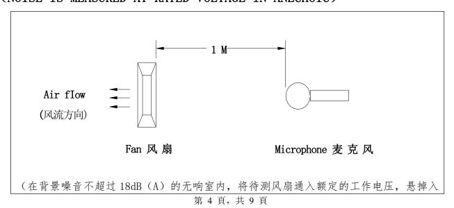
空中,将麦克风放于风扇同一平面且离待测风扇进风口一米处进行测试其 B&K 值) Noise is measured rated voItage in free air in anechoic chamber with B&K sound IeveI meter with microphone at a distance of one meter from the fan intake. The background noise is 18Db(A) max。
