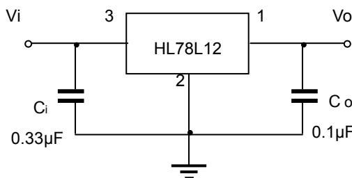
Note : Bypass capacitors are recommended for optimum stability and transient response and should be located as close as possible to the regulators.
