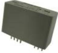
CSN Series closed loop current sensor, measures ac, dc or impulse current, 50 amp-turns nominal,  $\pm 90$  amp-turns range, miniature housing, 2000 turn
