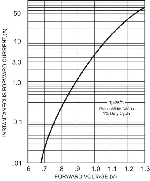
FIG.2-TYPICAL FORWARD CURRENT DERATING CURVE
