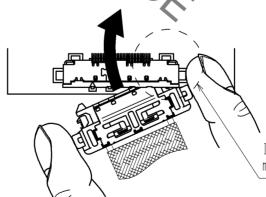
In case connector is withdrawn with lock that is locked on one side, mate the plug again and withdraw with <Correct withdrawal> method.
