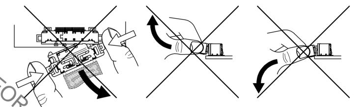
[4] For the case that connector is withdrawn in condition that lock on one side is locked
