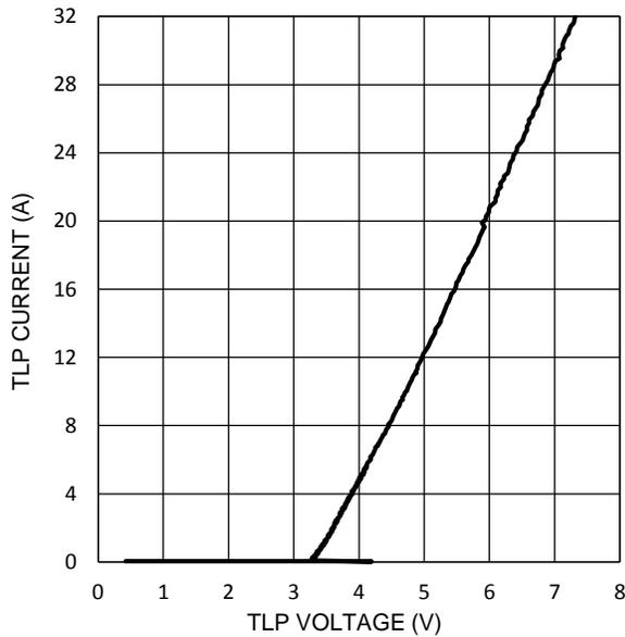
Figure 5 Pin 1 to Pin 2 TLP Curve ( $t_p = 100\text{ns}$ )
