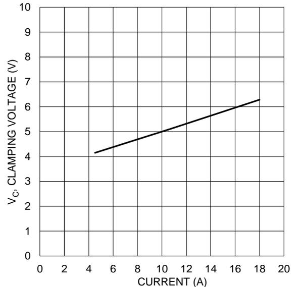
Figure 6 Clamping Voltage Characteristic ( $t_p = 8/20\mu\text{s}$ )
