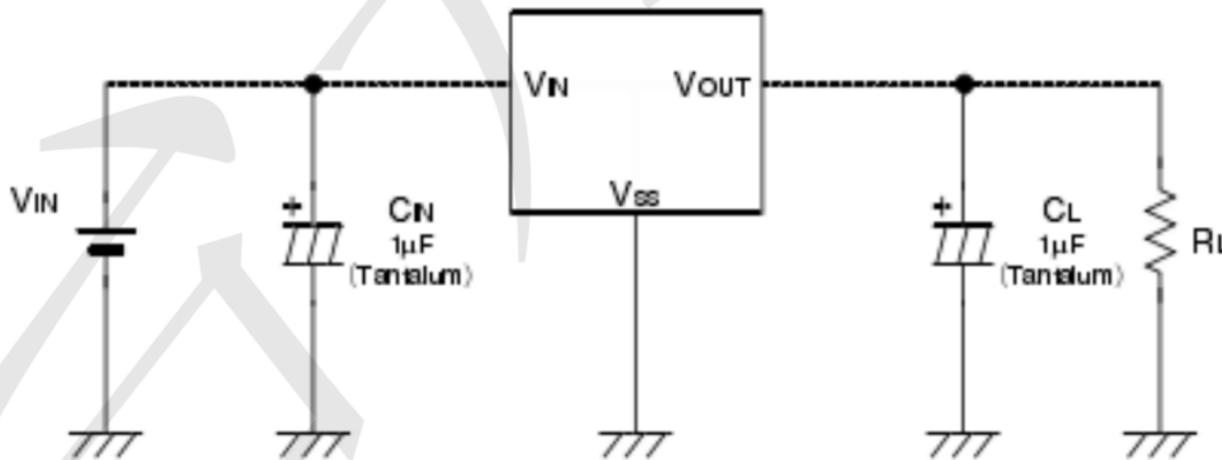
Note1: Input capacitor  $C_{IN}=1\mu F$ .
