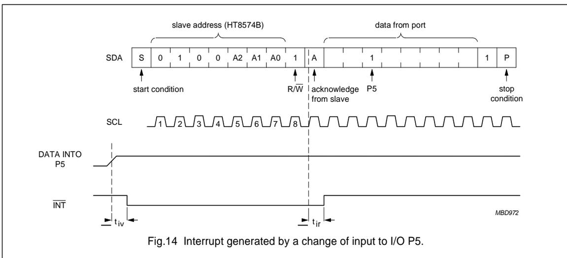
Fig.14 Interrupt generated by a change of input to I/O P5.
