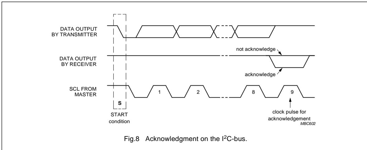
Fig.8 Acknowledgment on the I<sup>2</sup>C-bus.
