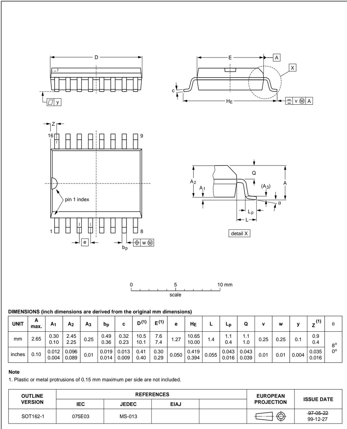
SSOP16: plastic small outline package; 16 leads; body width 3.9 mm
