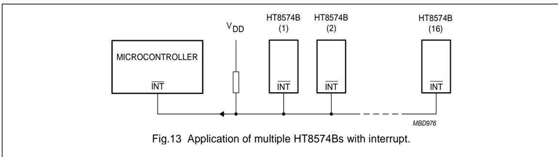
Fig.13 Application of multiple HT8574Bs with interrupt.
