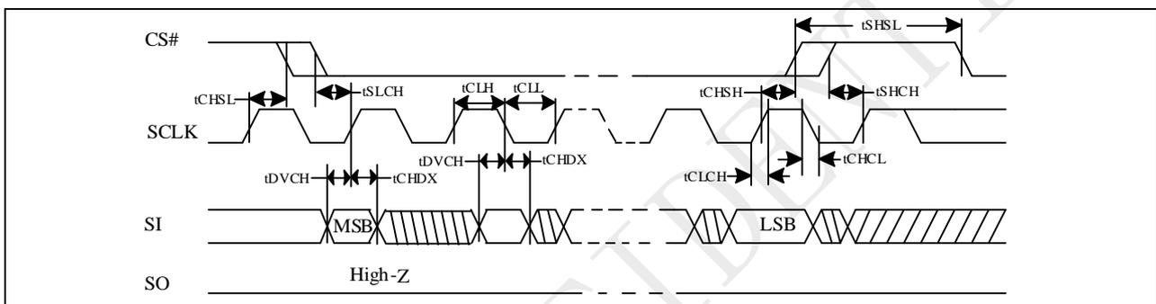
Figure 5-5 Output Timing
