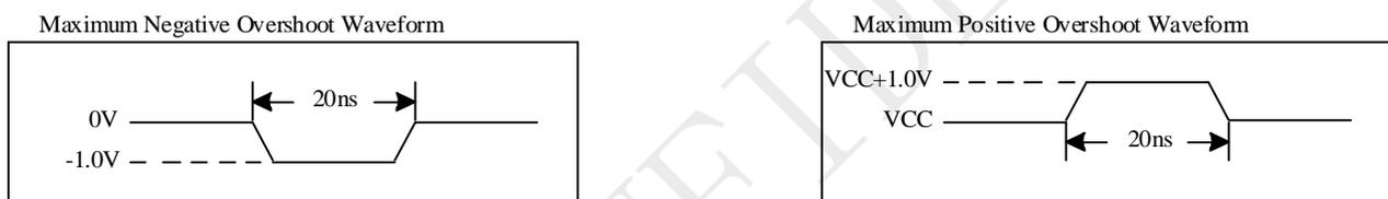
**Figure 5-2 Input Test Waveforms and Measurement Level**
