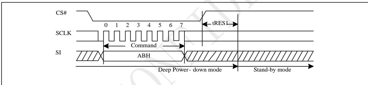
Figure 10-44c Release from Deep Power-down (RDP) Sequence (QPI)
