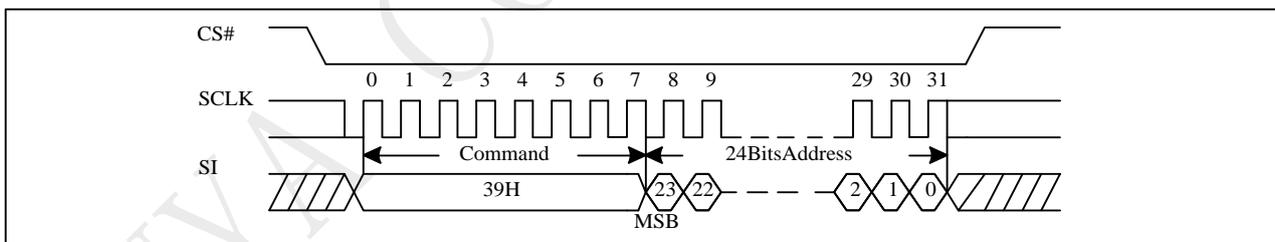
Figure 10-54 Individual Block Unlock (QPI)
