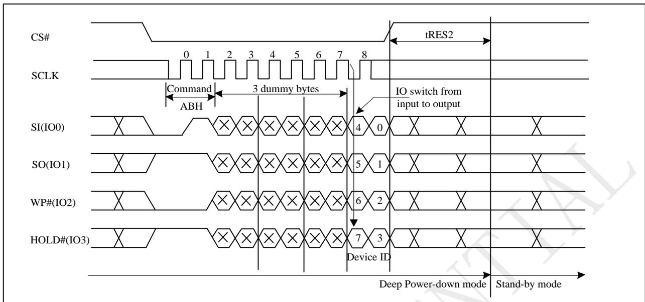
Figure 10-44b Release from Deep Power-down (RDP) Sequence (Command ABH)
