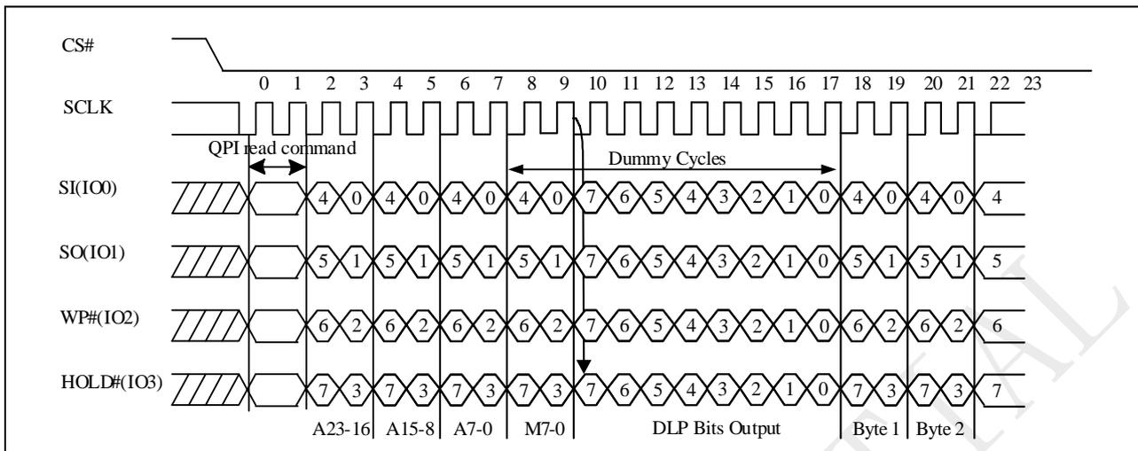
Figure 10-25e DTR 1IO Read with DLP bits output Sequence
