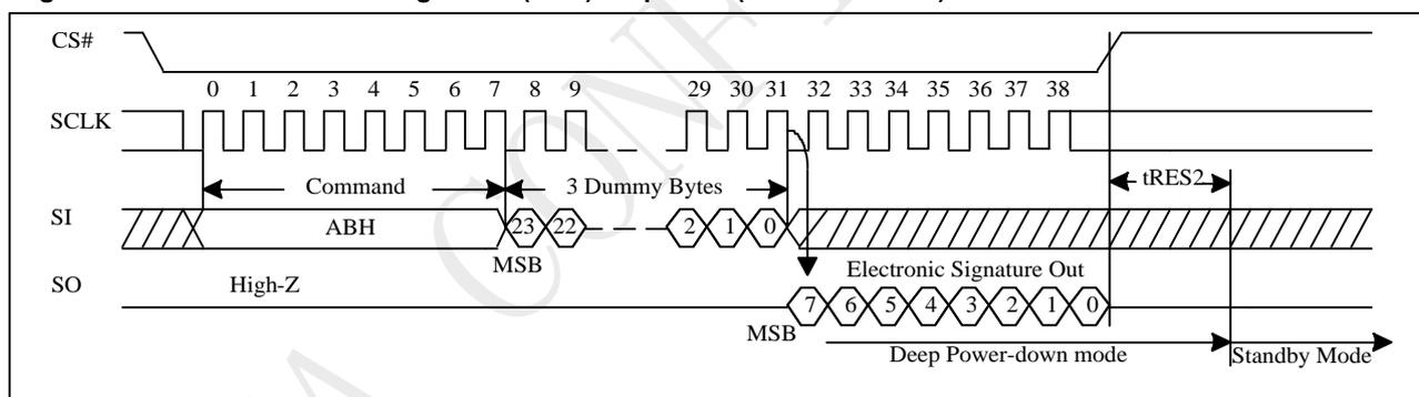
Figure 10-44a Read Electronic Signature (RES) Sequence (QPI)
