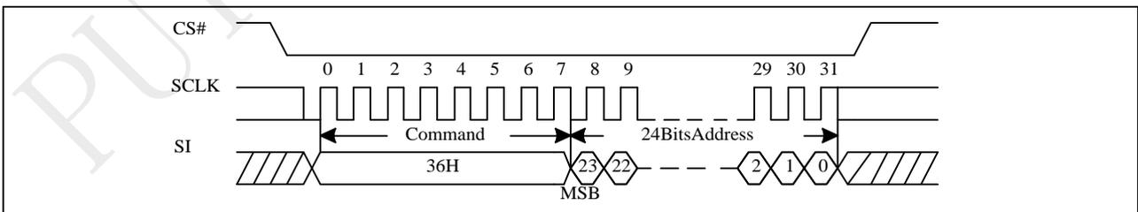
Figure 10-53 Individual Block Lock (QPI)
