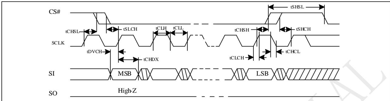
Figure 5-4b Serial Input Timing in DTR Mode
