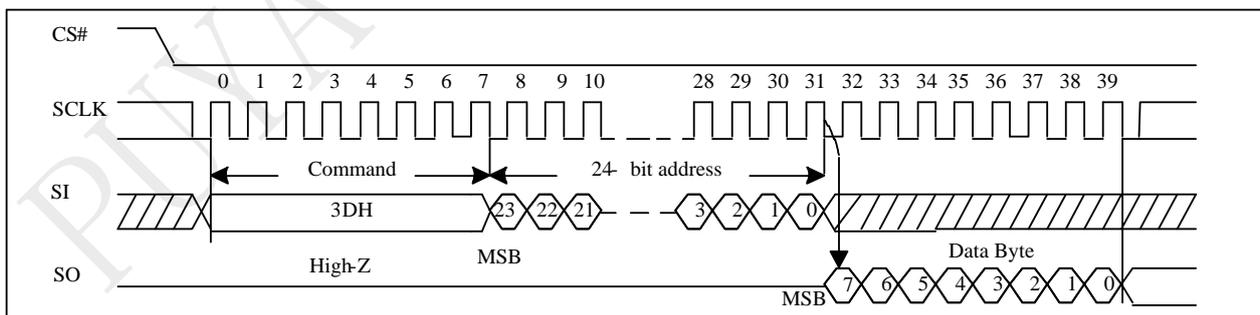
Figure 10-55a Read Block Lock Status (QPI)
