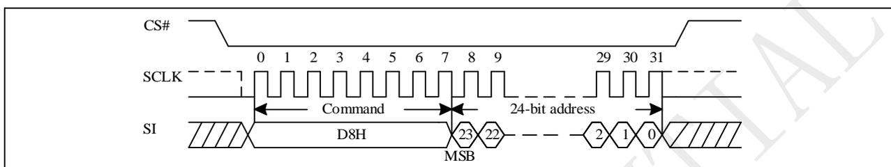
**Figure 10-31a Block Erase (BE) Sequence (QPI)**
