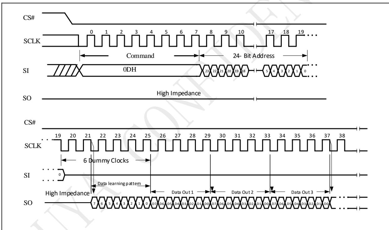
Figure 10-25e DTR 2IO Read with DLP bits output Sequence
