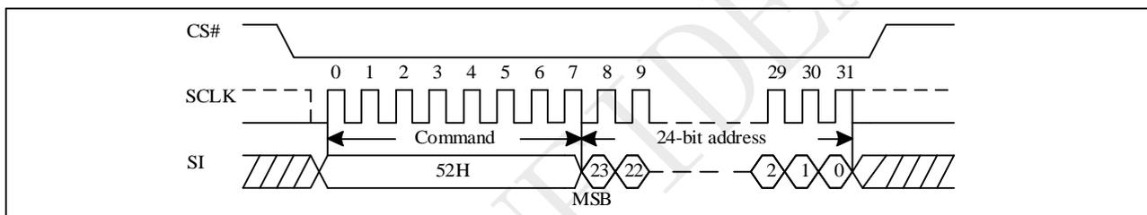
Figure 10-30a Block Erase 32K (BE32K) Sequence (QPI)
