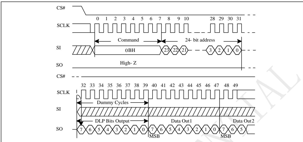
Figure 10-25a Dual Read with DLP bits output Sequence
