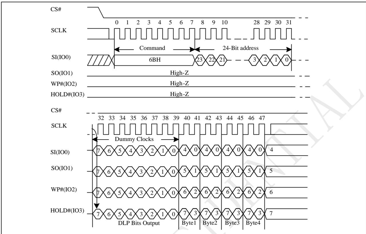
Figure 10-25c 4IO Read with DLP bits output Sequence
