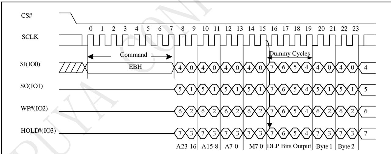
Figure 10-25d QPI Read instructions with DLP bits output Sequence
