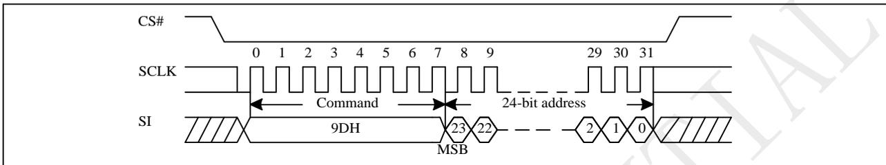
**Figure 10-39a Buffer to Main Memory Page Program Sequence (QPI)**
