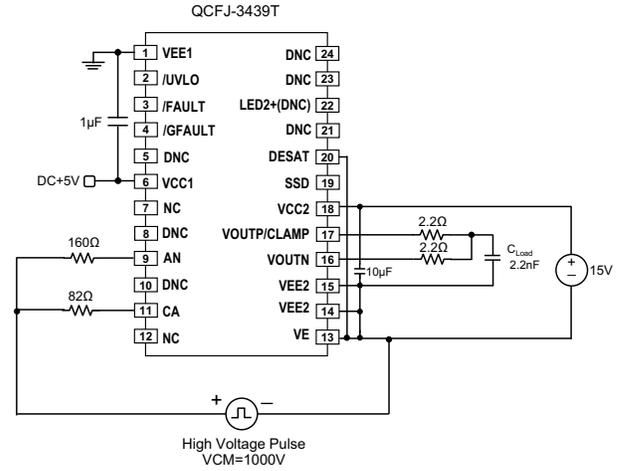
Figure 23: QCFJ-3439T Typical Gate Driver Circuit with IGBT Desaturation/Short-Circuit Sensing
