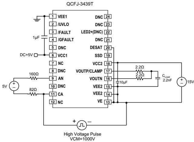
Figure 22: CMR Output Low Test Circuit
