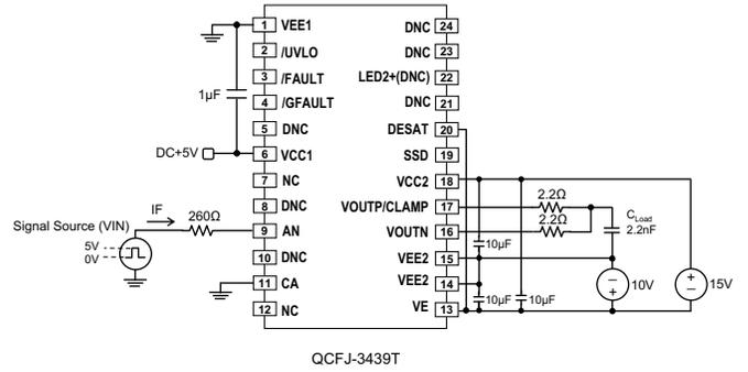
Figure 21: CMR Output High Test Circuit
