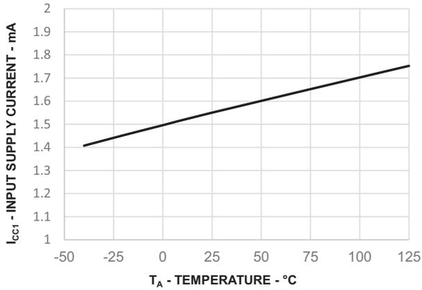
Figure 8:  $I_{CC2}$  vs. Temperature
