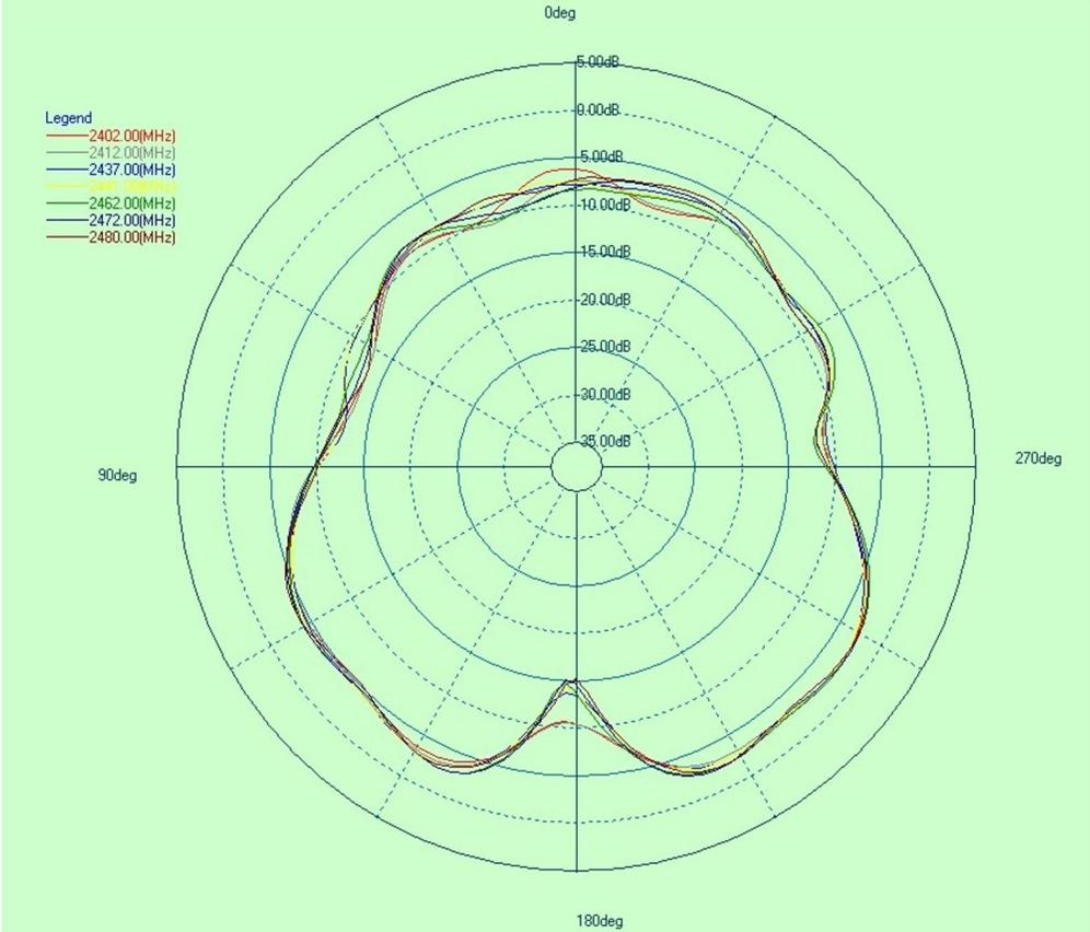
Figure 13-5. Antenna Radiation Pattern When Theta = 90 Degrees
