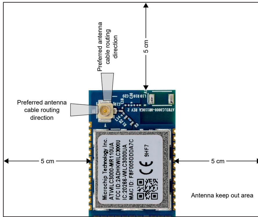
**Note:** These are generic guidelines and it is recommended that customers check and fine-tune the antenna positioning in the final host product based on RF performance.
