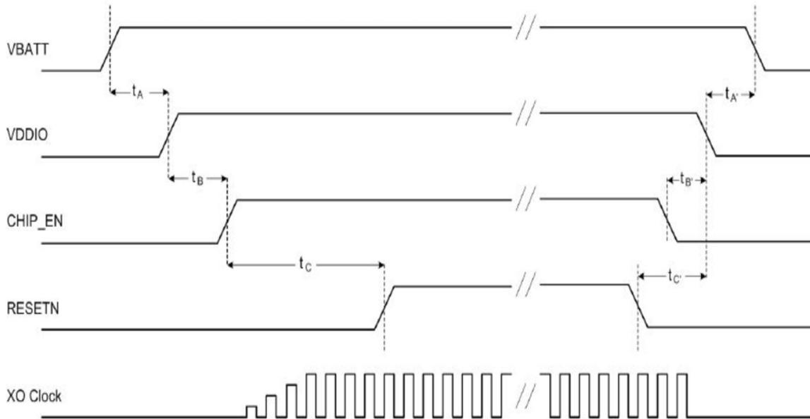
The following table provides power-up/down sequence timing parameters.
