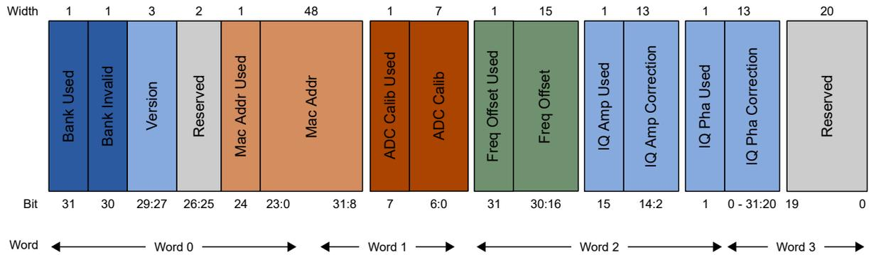
**Note:** The bit map was updated with bit fields IQ Amp correction and IQ Pha Correction fields from the firmware version 15.3 for WILC Linux and 4.5 for WILC RTOS onwards. Earlier, these bit fields were reserved for future use. For customers using firmware older than 15.3 for WILC Linux and 4.5 for WILC RTOS, IQ Amp correction and IQ Pha Correction bit fields will not be used by the firmware.
