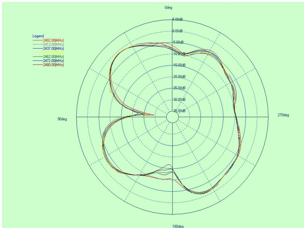
Figure 13-4. Antenna Radiation Pattern When Phi = 90 Degrees
