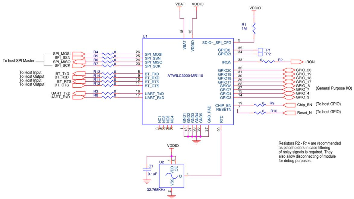
**Note:** Adding test points for module pins 8, 9, 10, 11, 16 and 17 in the design is recommended.
