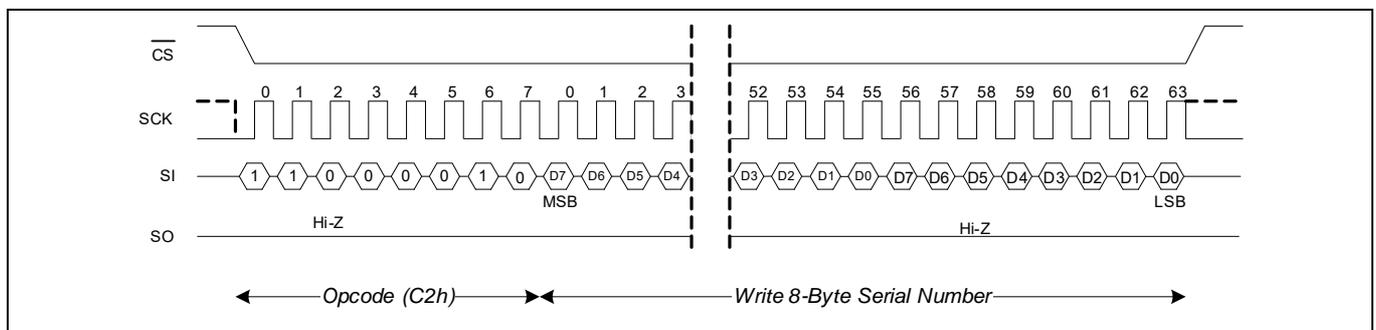
**Figure 17 Write serial number (WREN not shown) operation**
