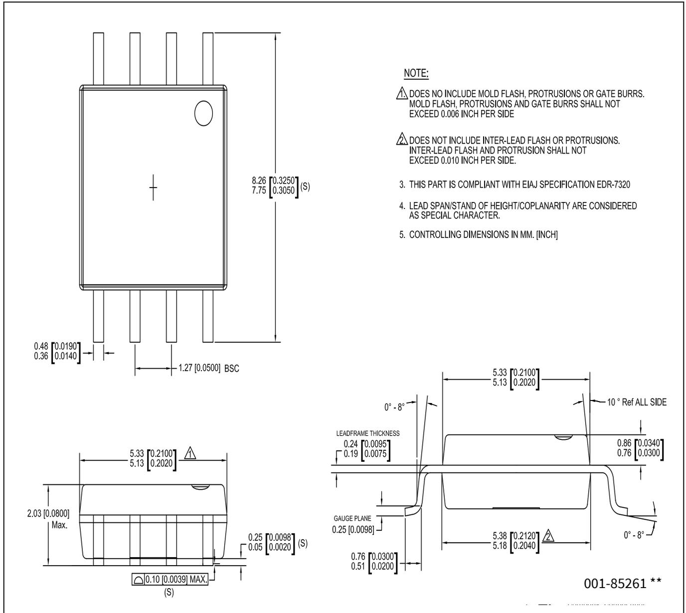
**Figure 25 8-pin SOIC (208 Mils) package outline, 001-85261**
