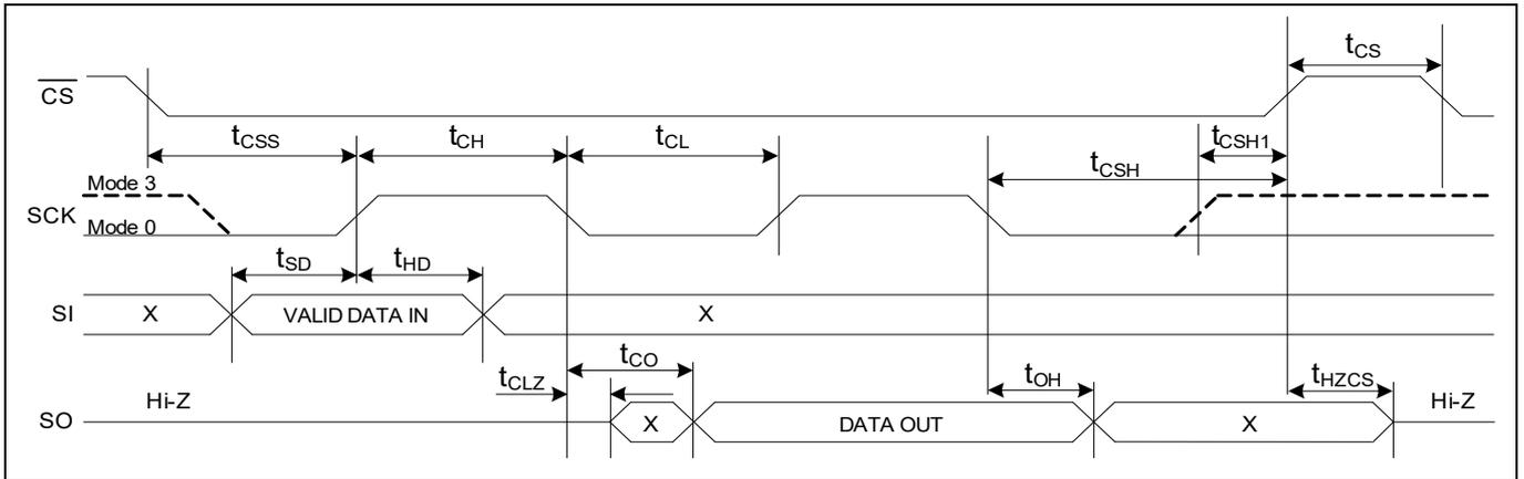
**Figure 22 Synchronous data timing (mode0 and mode 3)**
