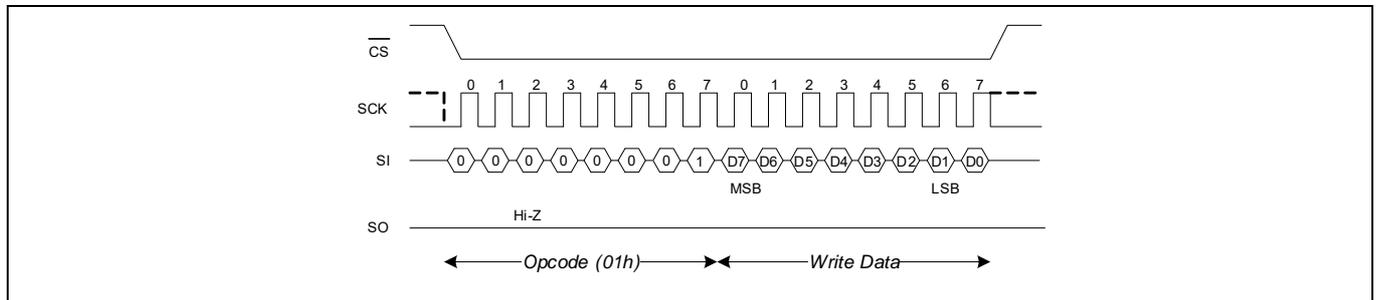
**Figure 9 WRSR bus configuration (WREN not shown)**
