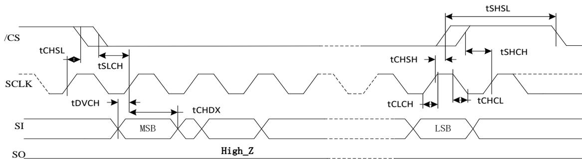
Figure 47. Output Timing
