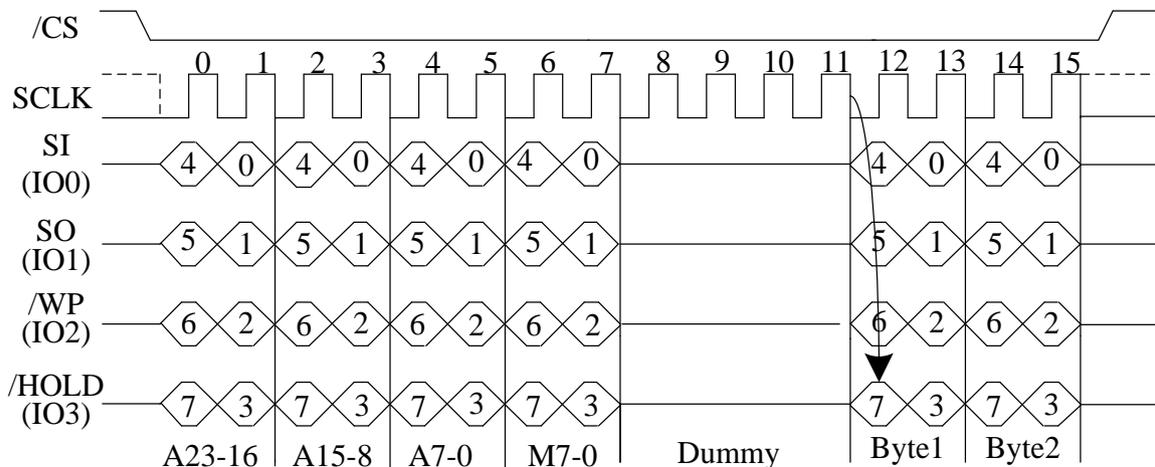
**Quad I/O Fast Read with “8/16/32/64-Byte Wrap Around”**
