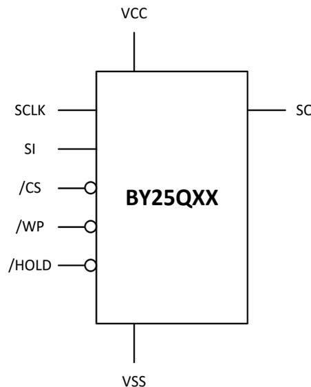
Figure 2. Pin Configuration SOP8
