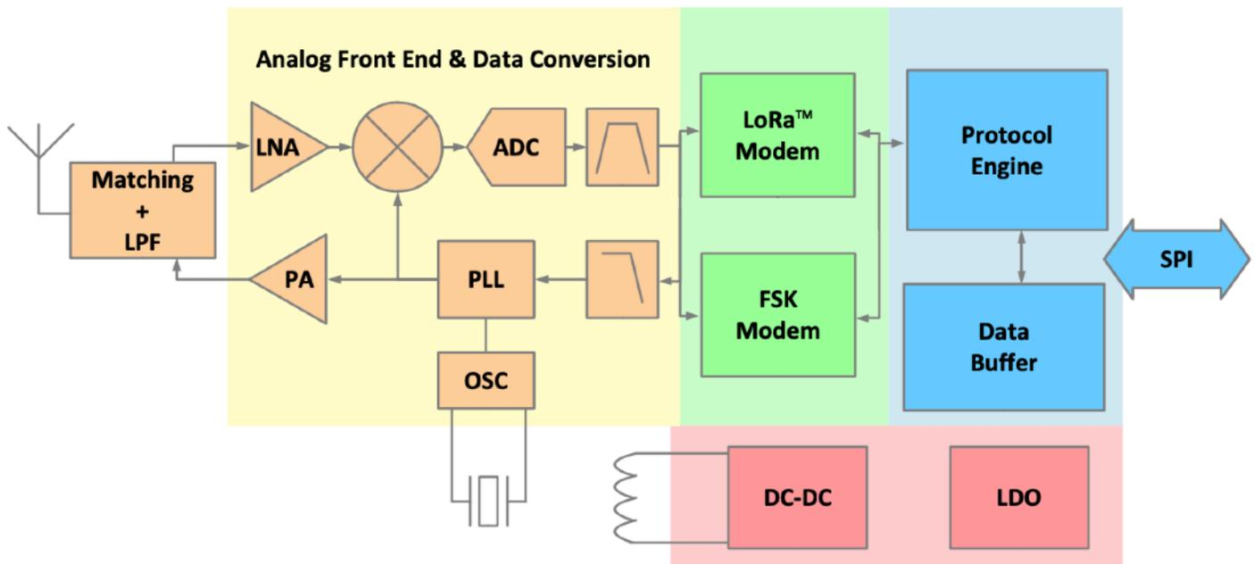
LR62E module has an u.FL connector for external antenna. In application example, a BM833 BLE module with Cortex M4F MCU manages LR62E through SPI interface.
