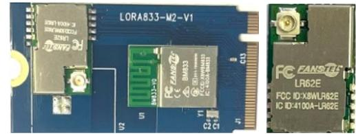
BM833 + LR62E pair can be used in LoRaWAN™ application. LoRaWan stacks are not available from Fanstel.
