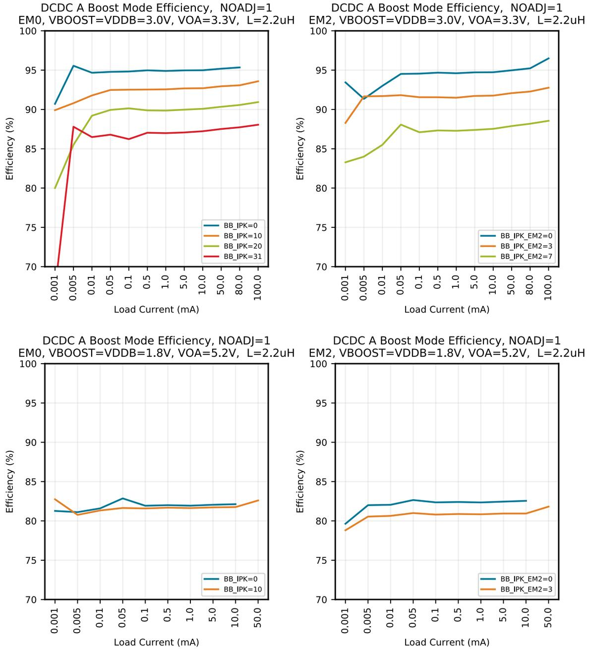
**Figure 5.12. Typical DCDC A Boost Efficiency, VOA=5.2V, NOADJ=1**
