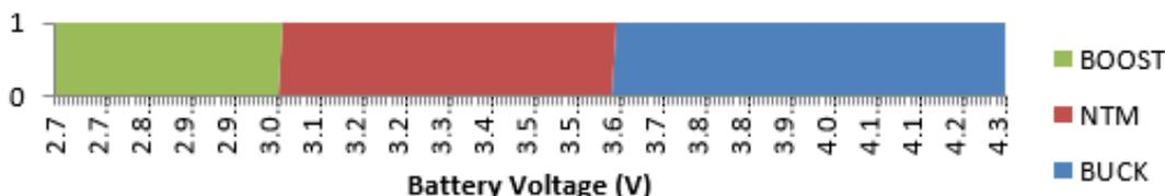
Figure 3.4. Operating Mode vs Battery Voltage, NTM\_LDO\_THRSH=3
