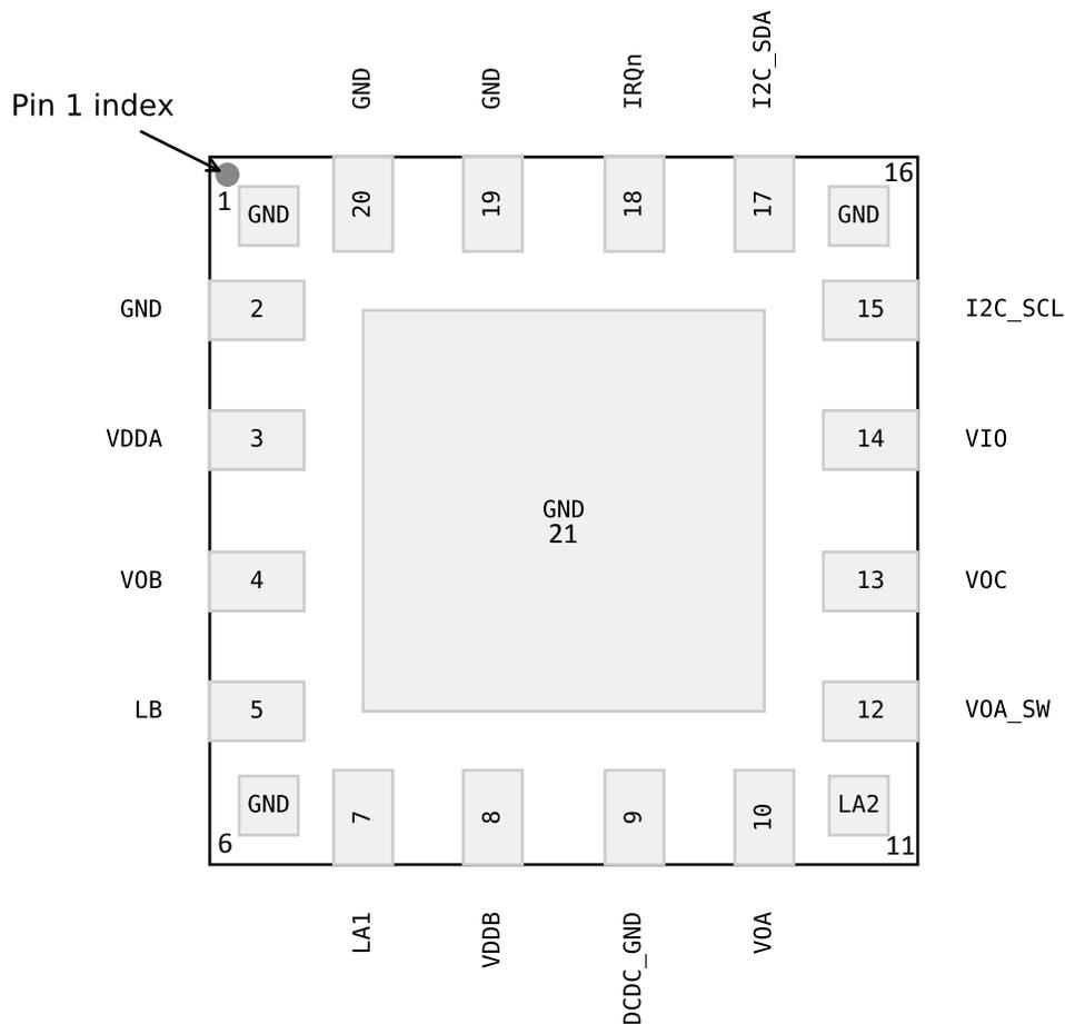
**Figure 8.1. EFP01 Device Pinout (Top View)**
