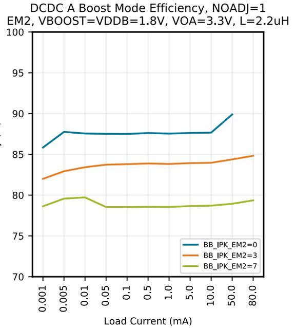
Figure 5.9. Typical DCDC A Boost Efficiency, VOA=3.3V, NOADJ=1
