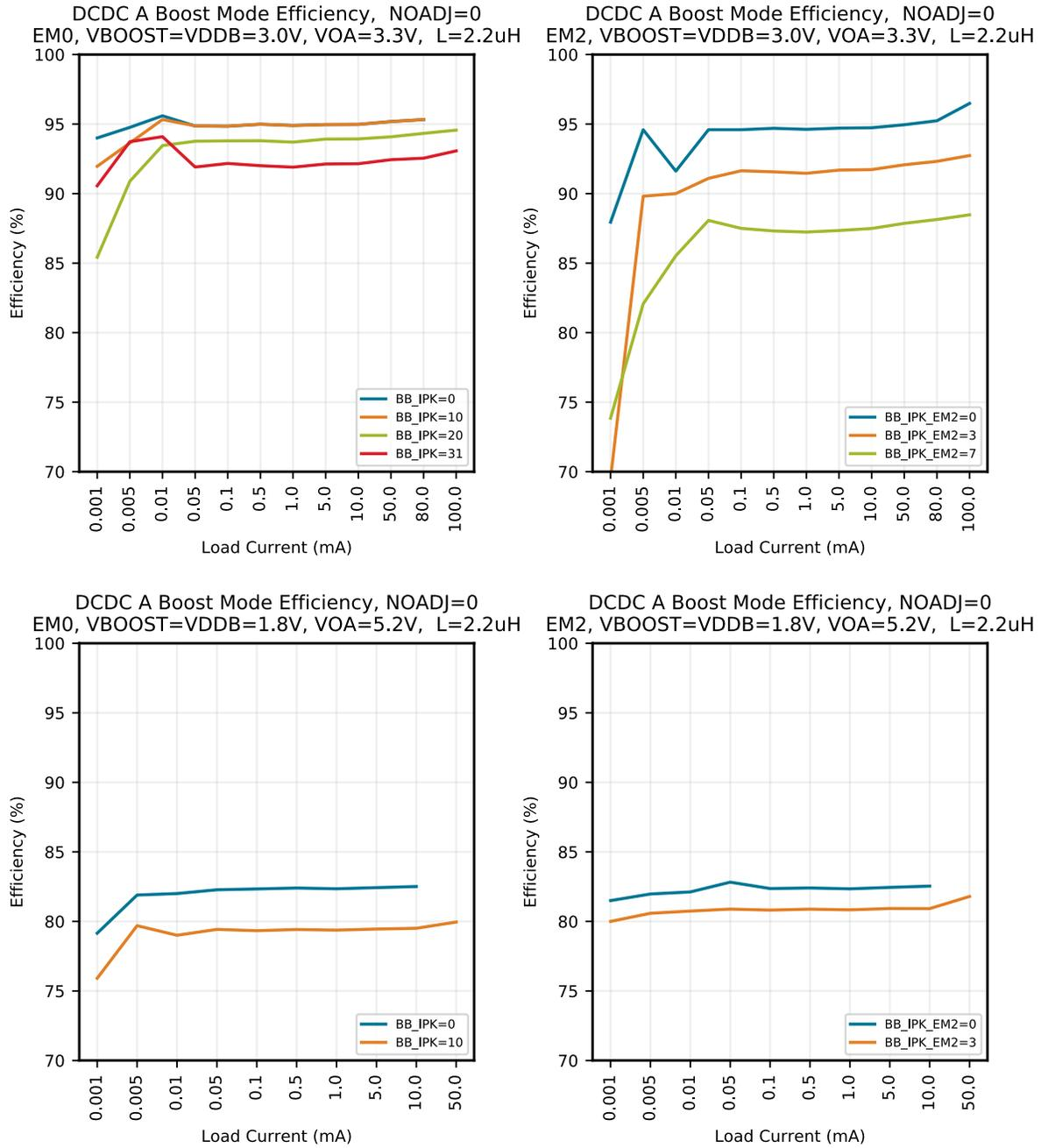
**Figure 5.6. Typical DCDC A Boost Efficiency, VOA=5.2V, NOADJ=0**
