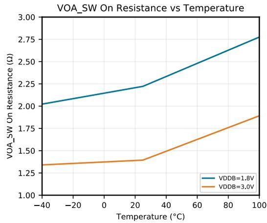
**Figure 5.15. Typical VOASW RDS ON vs Temperature**
