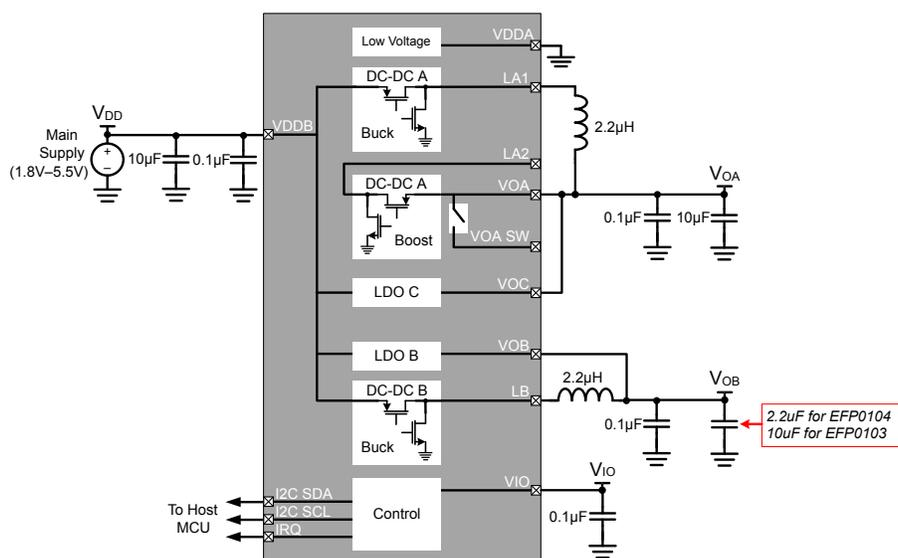
**Figure 4.2. Wired Buck with LDO C Configuration**
