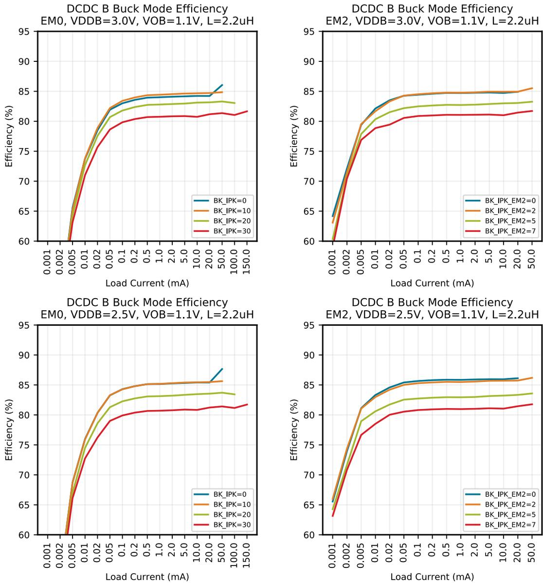
Figure 5.8. Typical DCDC B Buck Efficiency
