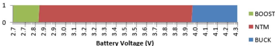
Figure 3.6. Operating Mode vs Battery Voltage, NTM\_LDO\_THRSH=7
