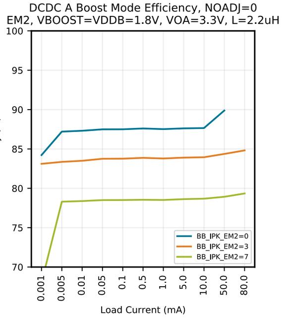
Figure 5.3. Typical DCDC A Boost Efficiency, VOA=3.3V, NOADJ=0
