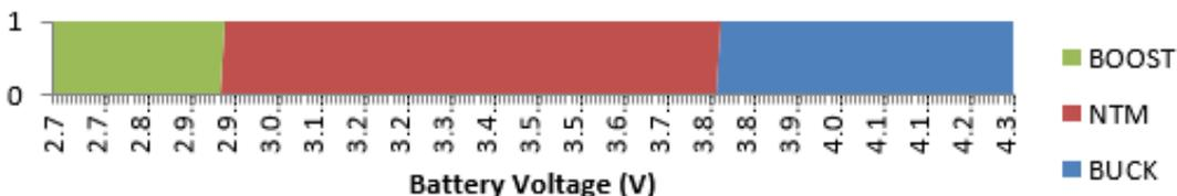
Figure 3.5. Operating Mode vs Battery Voltage, NTM\_LDO\_THRSH=5
