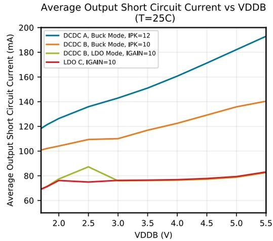
Figure 5.16. Typical Short Circuit Current vs VDDDB
