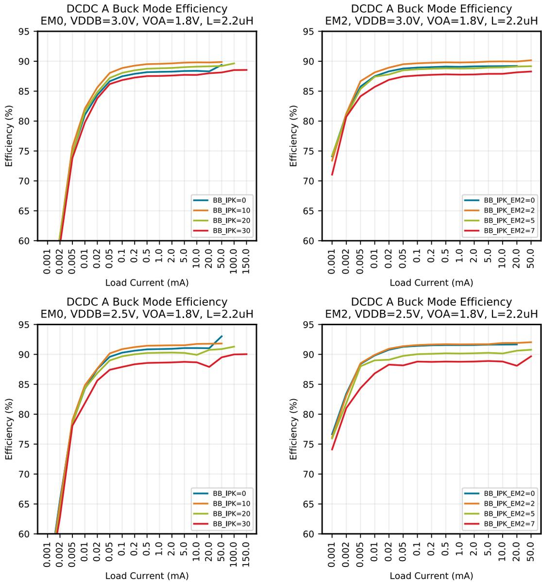
Figure 5.2. Typical DCDC A Buck Efficiency
