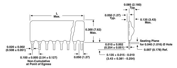
Pin #1 is extreme left-hand terminal on side with marking.
