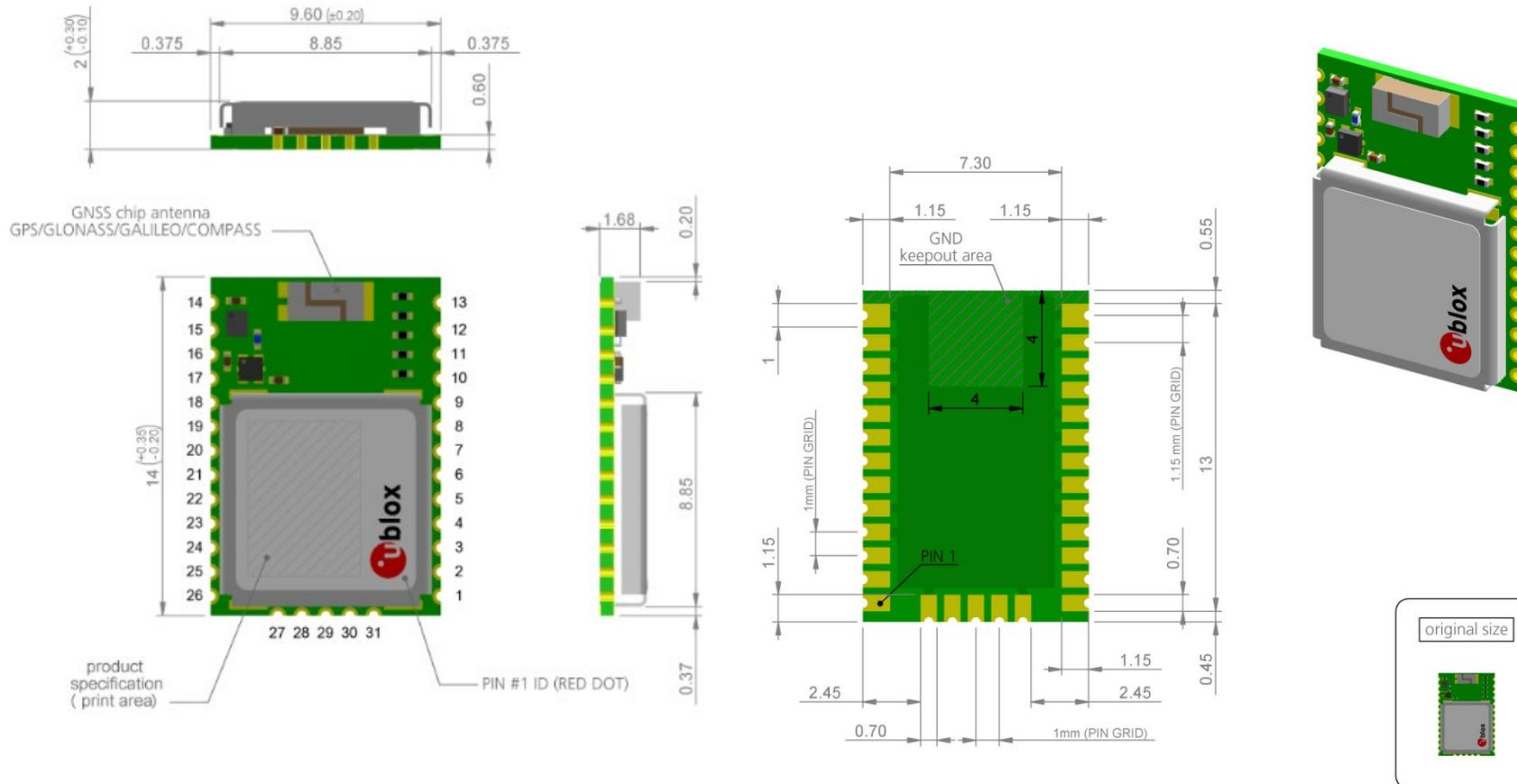
Figure 4: Dimensions (units: mm)
