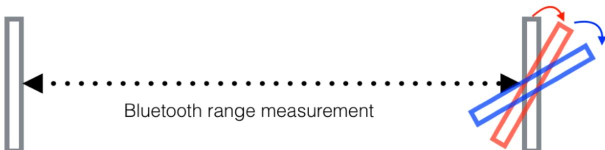
Bluetooth range is specified as the average of 12 measurements with the least significant digit truncated.
