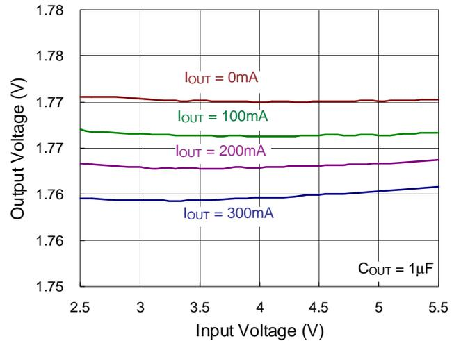
**LDO5 Output Voltage vs. Input Voltage**
