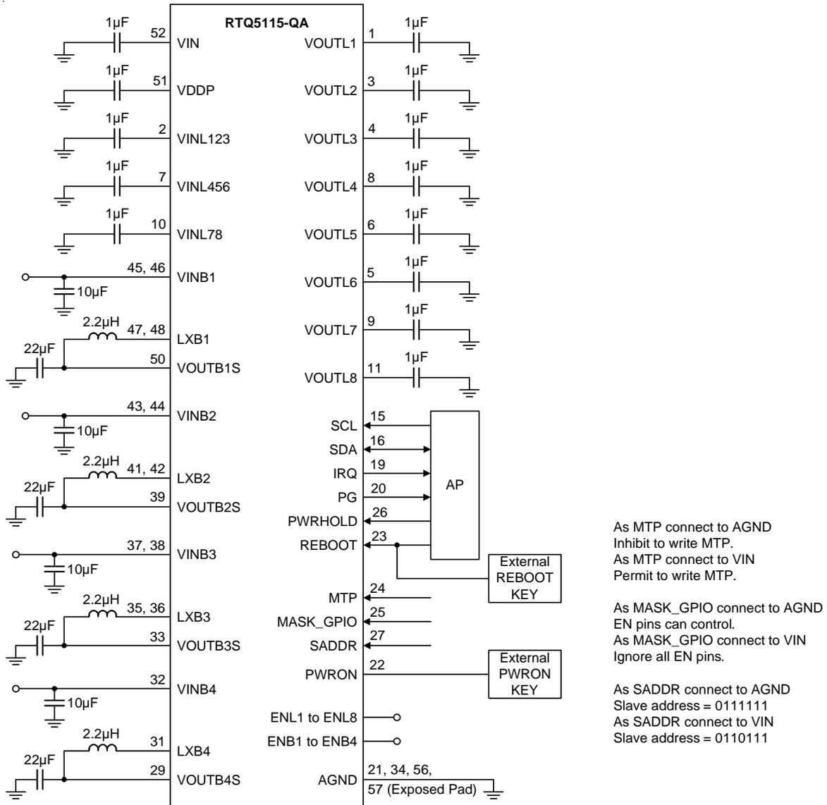
Suggested Components for Typical Application Circuit
