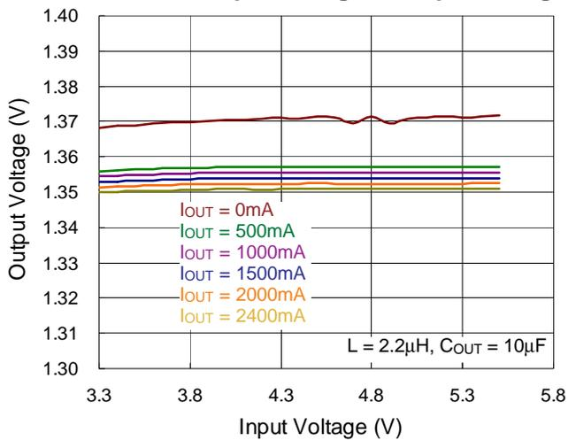
CH2 Buck Output Voltage vs. Input Voltage
