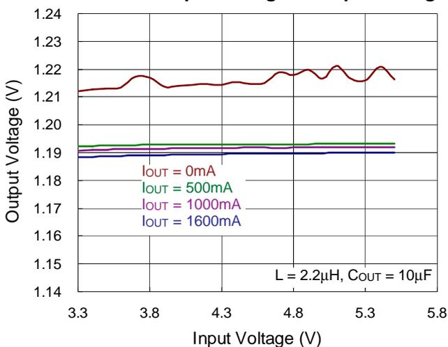
CH4 Buck Output Voltage vs. Input Voltage
