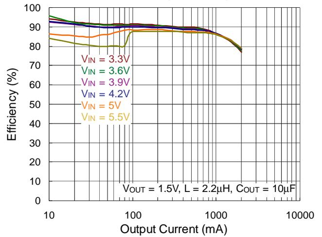
**CH3 Buck Efficiency vs. Output Current**
