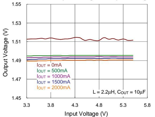
CH3 Buck Output Voltage vs. Input Voltage
