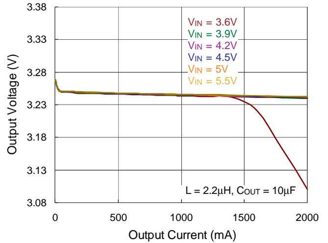
CH1 Buck Output Voltage vs. Input Voltage
