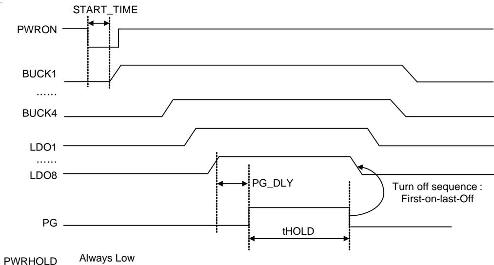
When AP sends the "PWRHOLD" signal during THOLD time, the RTQ5115 will keep power-on.
