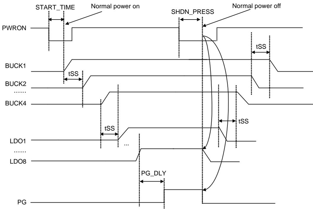
**Level Based ON/OFF Sequence (PWRON\_NORMOFF\_EN, Reg0x15[0] = 1)**
