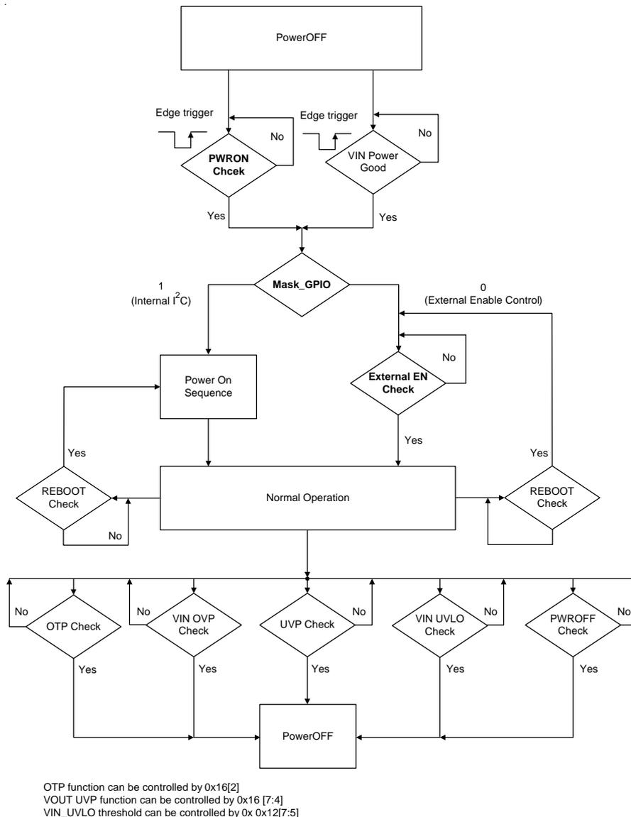
Figure 1. Power ON/OFF Flow Chart
