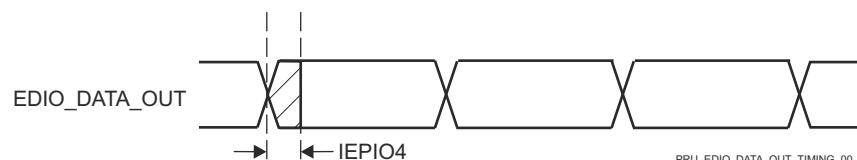
Figure 7-61. PRU-ICSS IEP Digital IOs Timing Requirements
