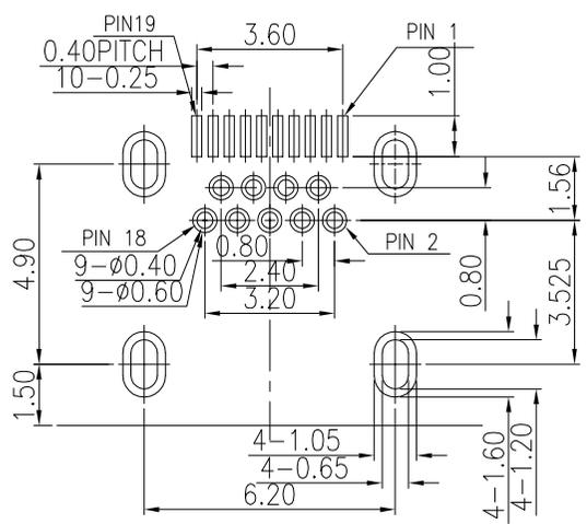
RECOMMENDED PCB LAYOUT THICKNESS = 0.8 mm
