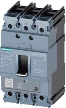
circuit breaker 3VA5 UL frame 125 breaking capacity class S 25kA @ 480 V 3-pole, line protection TM230, FTAM, In=50A overload protection Ir=50A fixed short-circuit protection Ii=5...10 x In cable connection on both sides
