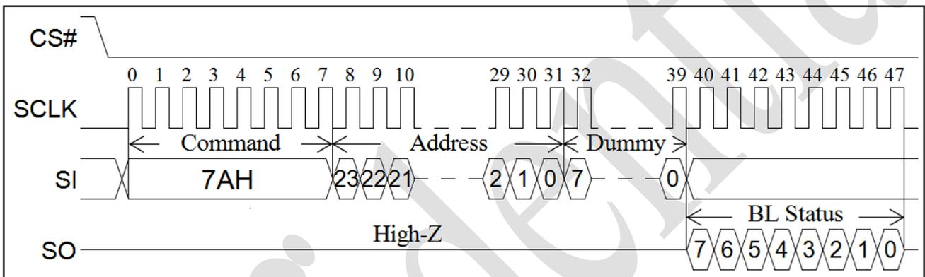
This register indicates whether a given block (addressed in the Block protection read address command field: BA[13:0]) is locked-down, locked or unlocked using the HWP or PBP).
