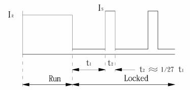
3rd wire signal Run : Square Wave Locked : Vhor VL
