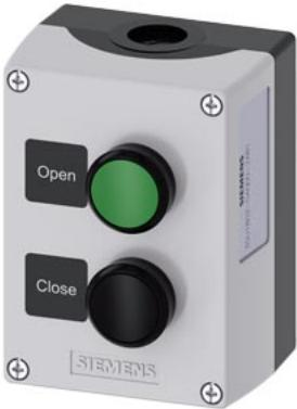
enclosure for command devices, 22 mm, round, enclosure material plastic, enclosure top part gray, 2 control points plastic, B=Pushbutton green, label: Open, 1 NO, screw terminal, A=Pushbutton black, label: Close, 1 NO, screw terminal, floor mounting, 1xM20 each on top and bottom, Labels glued in
