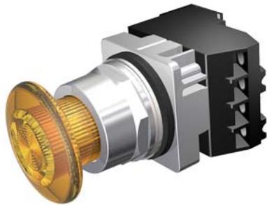
30mm Command/52, Chrome Finish Heavy Duty, Watertight/Oiltight Complete Metal Unit Illuminated Push-Pull Operator Transformer type, 600V AC Incandescent Lamp Mushroom Head Cap Small 1 3/4" (44.5 mm) Plastic, Amber 2 Position Maintained, Pull-to-Release with 1 N.O. - 1 N.C. Heavy Duty Contacts, A600/P600 UL Listed, CSA Certified NEMA 1,3,3R,4,4X,12,13 & Automotive Standards
