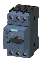
Special type Circuit breaker size S00 for transformer protection A-release 10...16 A N-release 286 A screw terminal Standard switching capacity Ambient temperature - 50 °C 500 switching cycles
