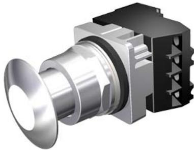
30mm Command/52, Chrome Finish Heavy Duty, Watertight/Oiltight Complete Metal Unit Illuminated Push-Pull Operator Full Voltage, 120V AC/DC Incandescent Lamp Mushroom Head Cap Small 1 3/4" (44.5 mm) Metal, Chrome with White Lens 2 Position Maintained, Pull-to-Release with 1 N.O. - 1 N.C. Heavy Duty Contacts, A600/P600 UL Listed, CSA Certified NEMA 1,3,3R,4,4X,12,13 & Automotive Standards
