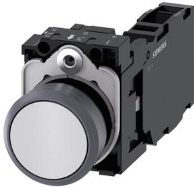
Pushbutton, 22 mm, round, plastic with metal front ring, white, pushbutton, flat, momentary contact type, with holder, 1 NO+1 NC, screw terminal
