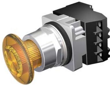
30mm Command/52, Chrome Finish Heavy Duty, Watertight/Oiltight Complete Metal Unit Illuminated Push-Pull Operator Transformer type, 120V AC Incandescent Lamp Mushroom Head Cap Small 1 3/4" (44.5 mm) Plastic, Amber 2 Position Maintained, Pull-to-Release with 1 N.O. - 1 N.C. Heavy Duty Contacts, A600/P600 UL Listed, CSA Certified NEMA 1,3,3R,4,4X,12,13 & Automotive Standards
