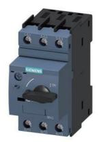
Circuit breaker size S0 For system protection Without phase failure protection A-release 18...25 A Short-circuit release 325 A Screw terminal Standard switching capacity
