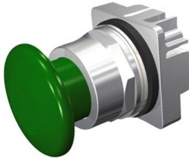
30mm Command/52, Chrome Finish Heavy Duty, Watertight/Oiltight Metal Operator, Round Push-Pull Operator Non-illuminated Mushroom Head Cap Small 1 3/4" (44.5 mm) Plastic, Green 2 Position Maintained, Pull-to-Release UL Listed, CSA Certified NEMA 1,3,3R,4,4X,12,13 & Automotive Standards
