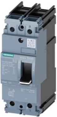
circuit breaker 3VA5 UL frame 125 breaking capacity class S 25kA @ 480 V 2-pole, line protection TM210, FTFM, In=80A overload protection Ir=80A fixed short-circuit protection li=10 x In UL489 SB (naval), 50 deg. cel. cable connection on both sides
