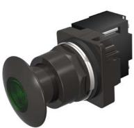
30mm BlackMax, Epoxy Coated Corrosion Resistant Complete Metal Unit Illuminated Push-Pull Operator Full Voltage, 6V AC LED Lamp Mushroom Head Cap Small 1 3/4" (44.5 mm) Metal, Black with Green Lens 3 Position Pull-Momentary/Push-Maintained UL Listed, CSA Certified NEMA 1,3,3R,4,4X,12,13 & Automotive Standards
