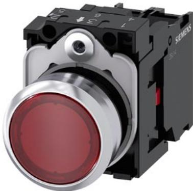
Illuminated pushbutton, 22 mm, round, metal, shiny, red, pushbutton, flat, momentary contact type, with holder, 1NC, LED module with integrated LED 24 V AC/DC, screw terminal, with laser labeling, upper case
