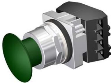
30mm Command/52, Chrome Finish Heavy Duty, Watertight/Oiltight Complete Metal Unit Push-Pull Operator Non-Illuminated Mushroom Head Cap Small 1.73" (44 mm) Metal, Anodized Green 3 Position Momentary 1 N.C.+1 N.C. Extra Late Break Heavy Duty Contacts, A600/P600 UL Listed, CSA Certified NEMA 1,3,3R,4,4X,12,13 & Automotive Standards
