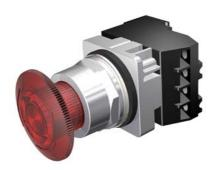
30mm Command/52, Chrome Finish Heavy Duty, Watertight/Oiltight Complete Metal Unit Illuminated Twist-to-Release Full Voltage, 6V AC LED Lamp Mushroom Head Cap Small 1.79" (45 mm) Plastic Cap, Red 2 Position Maintained, Twist-to-Release with 1 N.O. - 1 N.C. Heavy Duty Contacts, A600/P600 UL Listed, CSA Certified NEMA 1,3,3R,4,4X,12,13 & Automotive Standards
