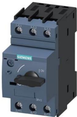
Circuit breaker size S0 For transformer protection A-release 2.8...4 A Short-circuit release 82 A Screw terminal Standard switching capacity
