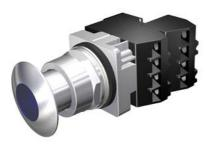
30mm Command/52, Chrome Finish Heavy Duty, Watertight/Oiltight Complete Metal Unit Illuminated Push-Pull Operator Full Voltage, 24V AC/DC Incandescent Lamp Mushroom Head Cap Small 1 3/4" (44.5 mm) Metal, Chrome with Blue Lens 3 Position Pull-Momentary/Push-Maintained 1 N.C.+1 N.C. Extra Late Break Heavy Duty Contacts, A600/P600 UL Listed, CSA Certified NEMA 1,3,3R,4,4X,12,13 & Automotive Standards
